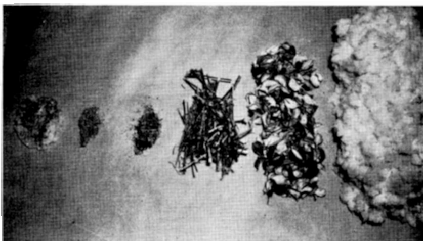
Figure 4. The composition of the harvested material. From left to right: Motes; small leaf trash; large leaf trash; sticks; burrs; and clean seed-cotton.
