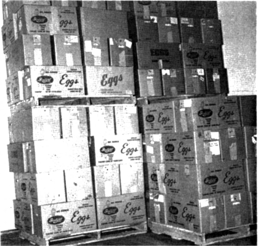
In models E and F pallets are stacked two high in the refrigeration rooms. High-piler fork-trucks are needed for the stacking, but refrigeration ownership and operating costs are lowered through use of high ceiling rooms.
