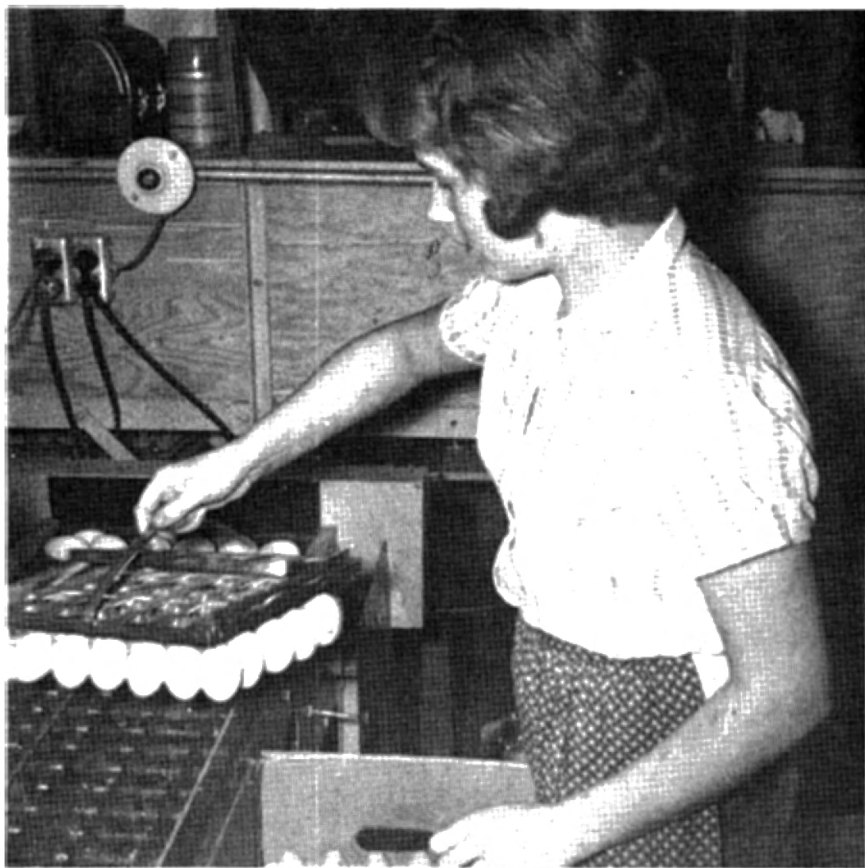
Mechanical lifters such as this one, and vacuum lifters of a similar type, are used in mass-candling operations. They quickly and easily move a layer of eggs from the case.
