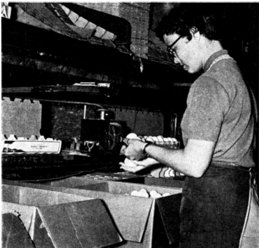
All six model plants have this type candling bench arrangement. Candler pulls in ungraded case and pushes out empty case.
