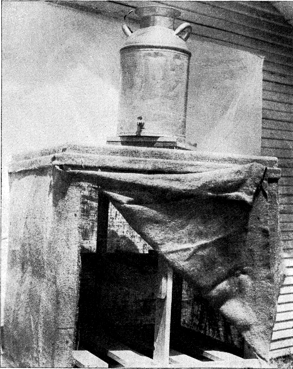
Figure 6.—Completed cooler, with pre-cooling compartment open. The cream can contains water which drips on cooler from faucet at base of can.
