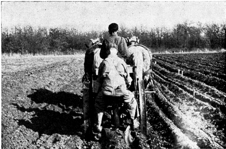
Fig. 9.—Potato planter with band fertilizer distributor in action. This is the machine shown close up in Figure 8.
