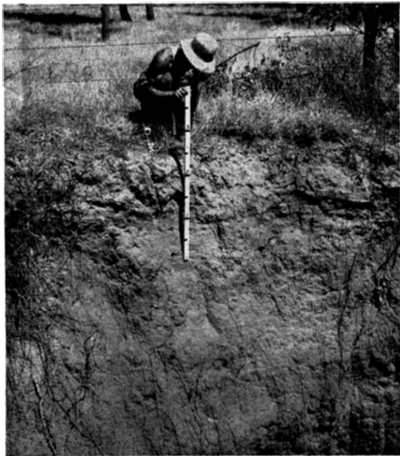
Figure 19. This particular soil has a deep, permeable profile which will absorb water readily.
