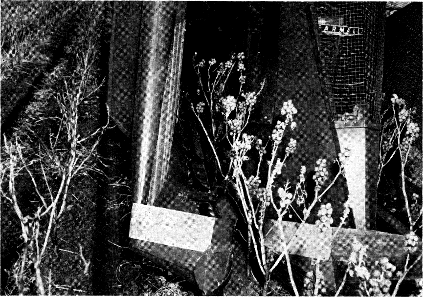
Fig. 5.—Harvester in operation stripping Cimarron variety castor beans which were about four feet tall and yielded approximately 900 pounds of seed per acre. The absence of leaves and weeds helps get clean beans in machine harvesting.
