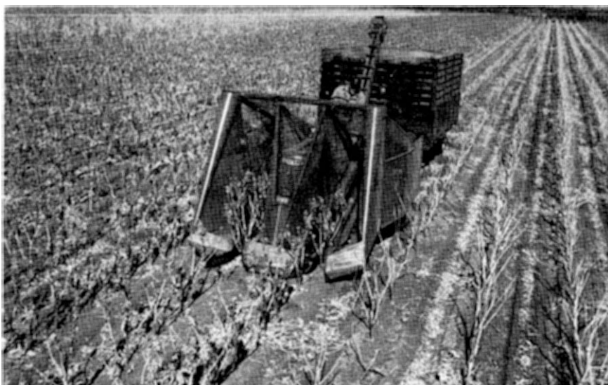
Fig. 12.—The two-row castor bean harvester in field operation.
