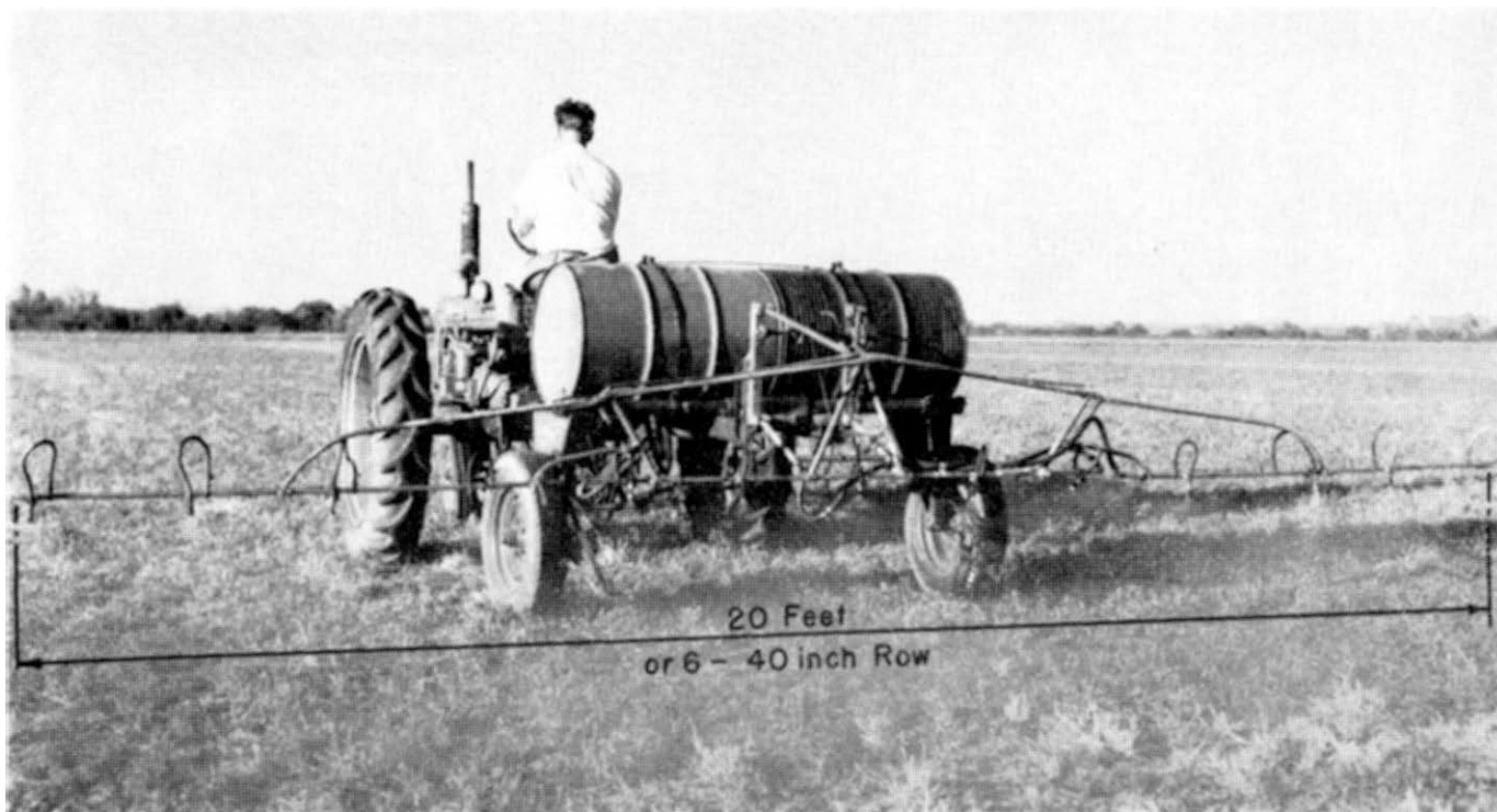
Fig. 7.—The spray boom is wide enough to cover a 20-foot swath in broadcast spraying, or six rows when working on row crops. Up to three nozzles per row are available to give thorough coverage.
