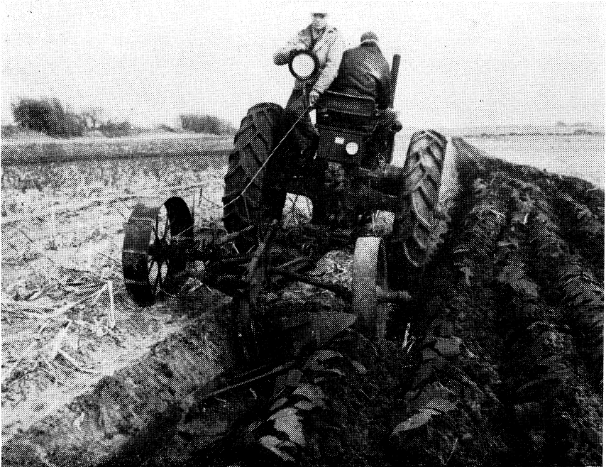
Fig. 9.—Moldboard Extension Controls Furrow Slice on 18-inch Plow.
