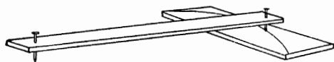
Figure 31—Marking off ribs for concrete silo forms, or for any other circular cuts requiring accuracy. Strings are not reliable
