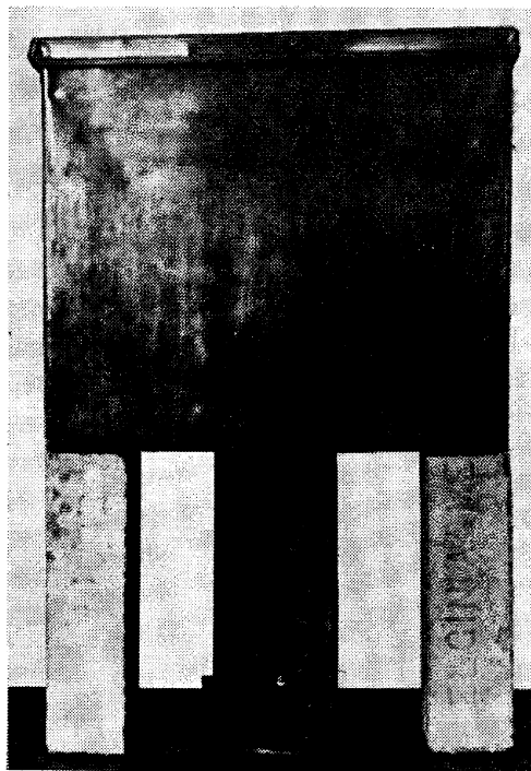
Figure 2. An inexpensive sterilizer for culture milk. The sterilizer is made of sheet copper and has a tight-fitting lid.
