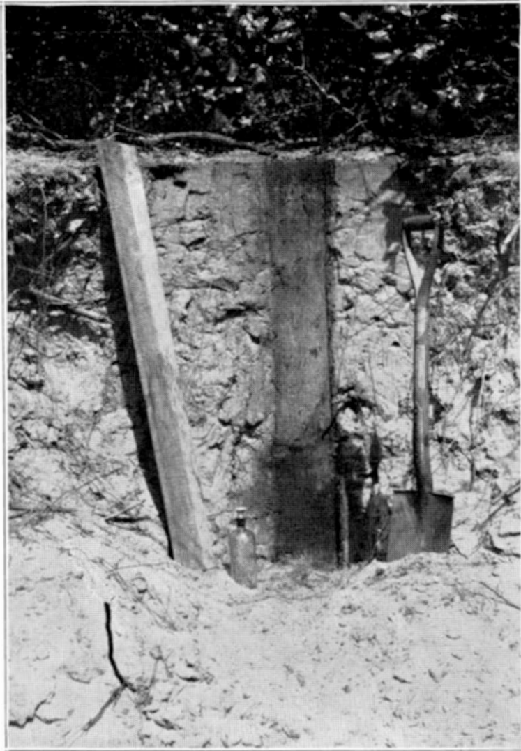
Fig. 1. Soil face recently treated with lacquer and smoothed so that board at left may be attached.
