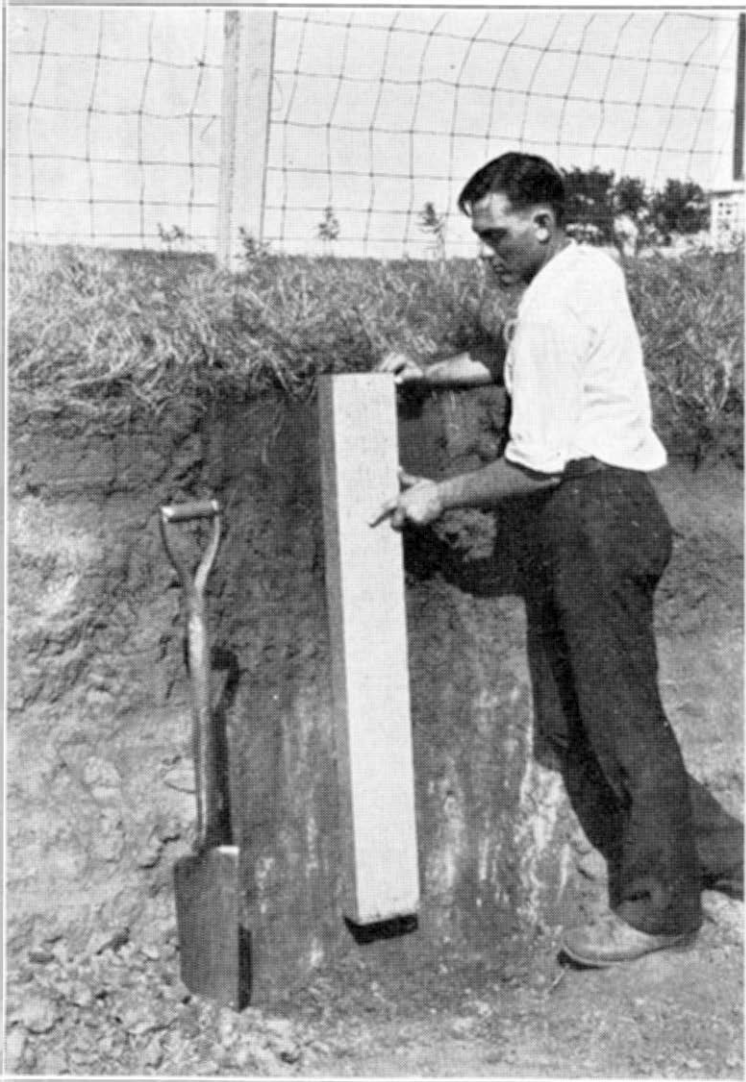
Fig. 3. The metal trough is ready to be forced into soil face, after which the profile will be transferred to the laboratory to be mounted.
