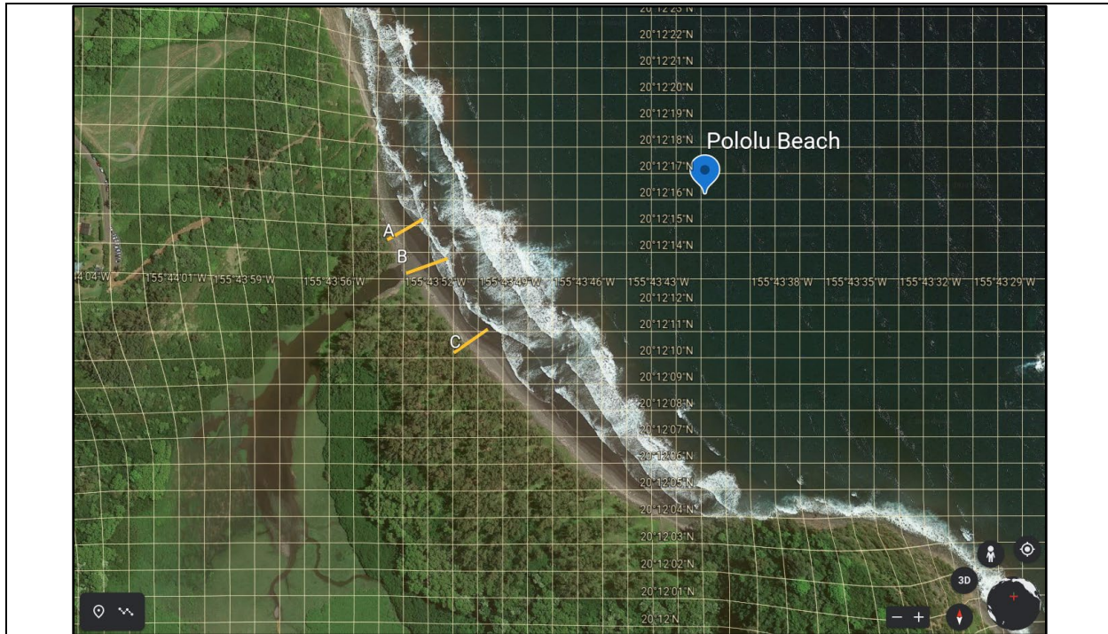
A.1.1: Pololu beach with corresponding transect locations. Number of transects: 3. Number of surveys: 14; A(1-4), B(1-3), C(1-7).
