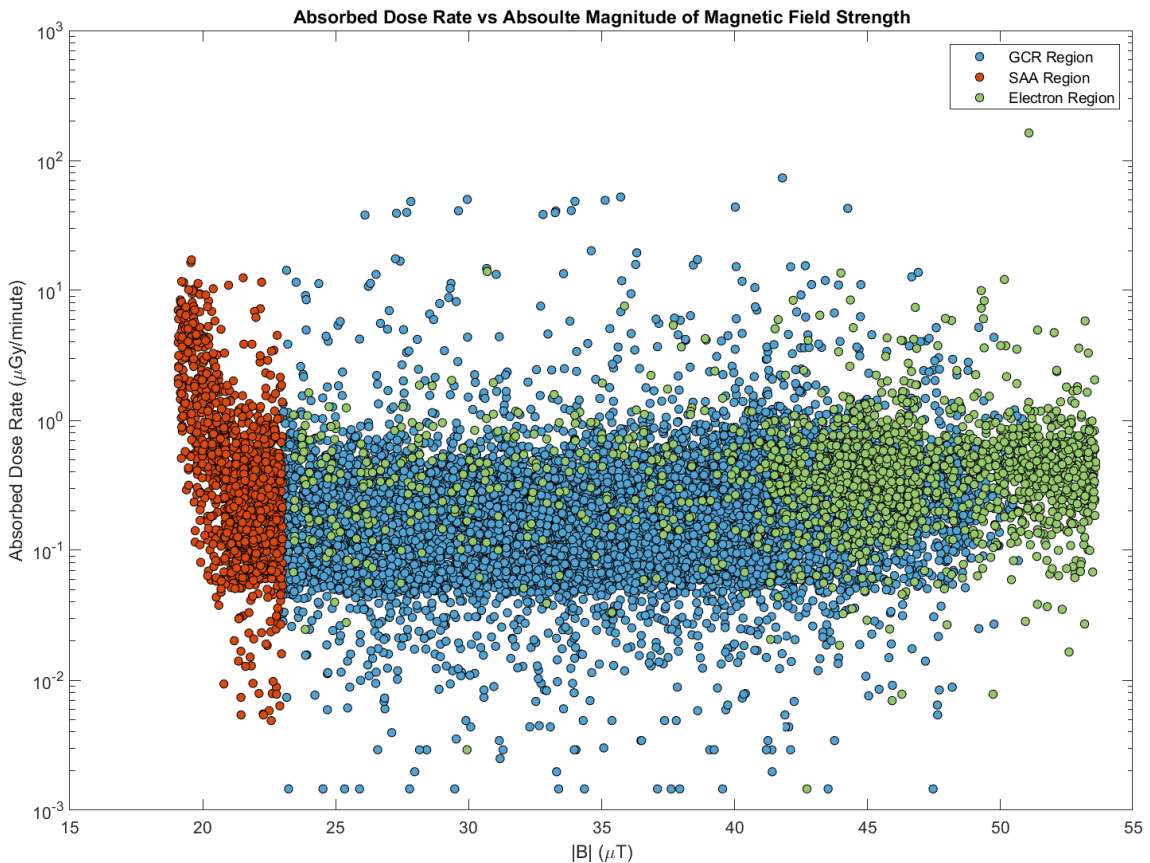
Figure 9.17: Absorbed dose rate as a function of magnetic flux density for region-separated ATED measurements aboard the ISS. Each region is color-coded to its corresponding region.
