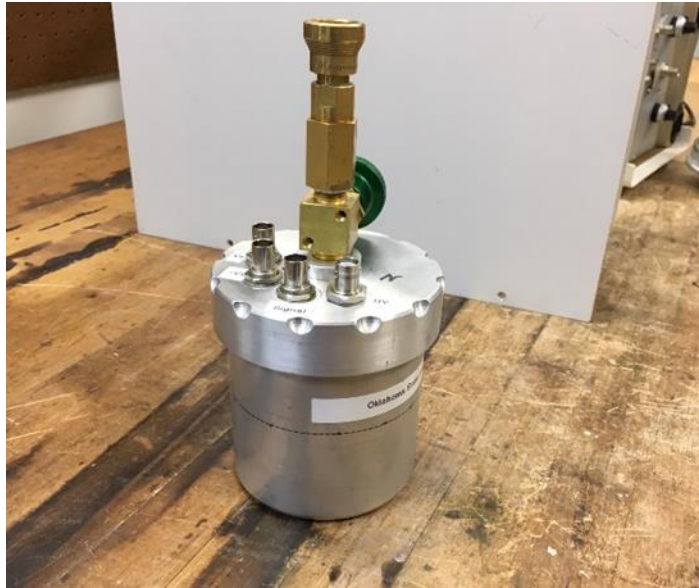
Figure 3.8 A re-sealable can with BNC and SHV feedthroughs. The large brass component is the valve which gas can be evacuated and refilled into the can. This older model of ATED detector head was fabricated by [Collums, 2012].
