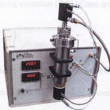
Figure 3.10: Automatic Klinkenberg permeameter/porosimeter (AP-608) for measuring sample porosity and permeability as a function of confining pressure up to 10, 000 psi.
