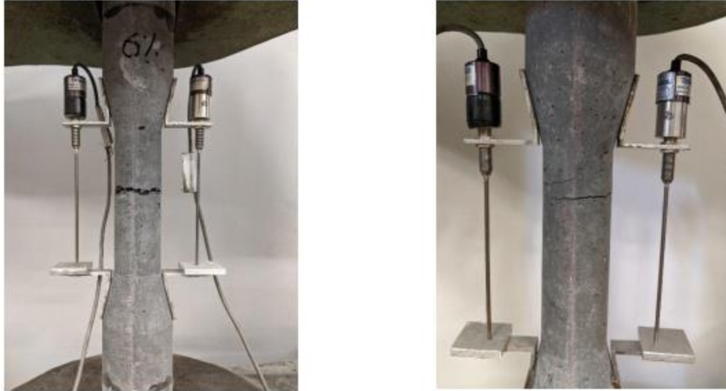
Figure 2.8 – Failed specimens with a single crack (left) and multiple cracks (right) (Lepissier, 2020)
