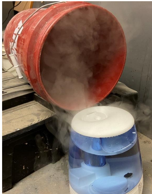
Figure 3.2 – Moist curing method for 0% specimens
