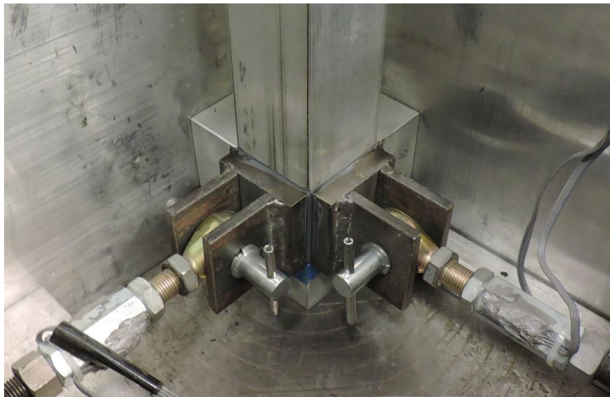
Figure 5.10 – Cube specimen with TTC fixtures in Looney Bin
