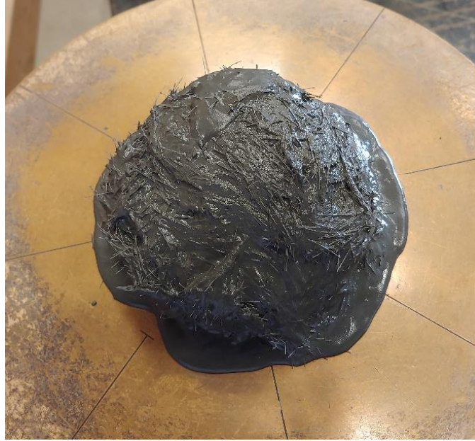
Figure 3.8 – Flow of the UHPC mix with 6% fibers
