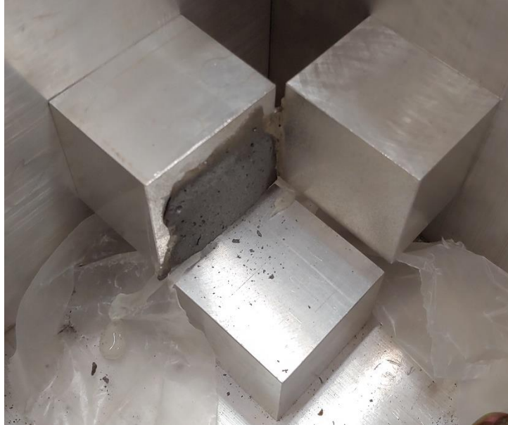
Figure 4.22 – Evidence of bond failure on plinths
