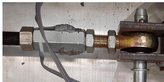
Figure 4.17 – Coupling nut load cell attached to test fixture
