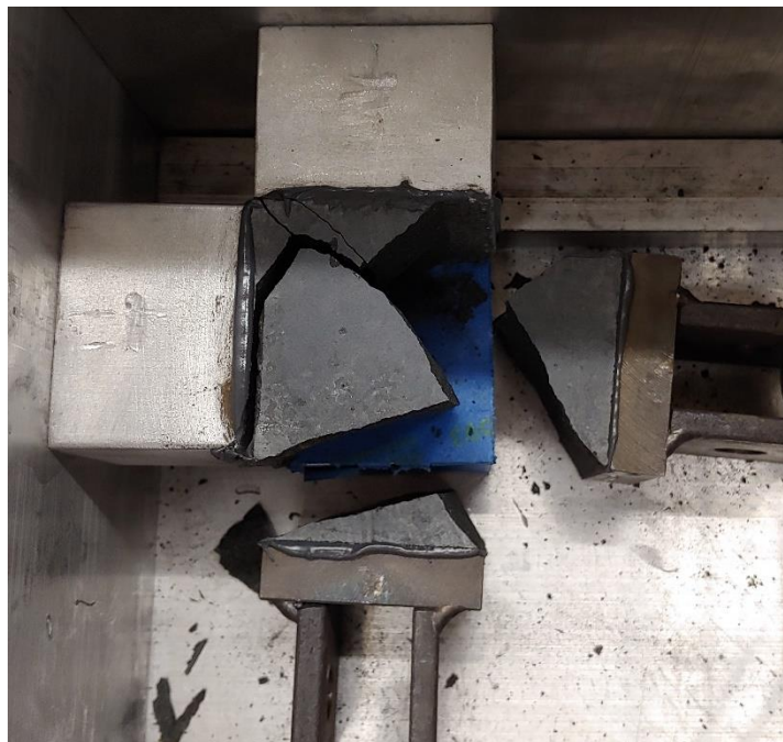
Figure 6.20 – Failed 0% fiber TT specimen subjected to proportional loading with substantial cracking
