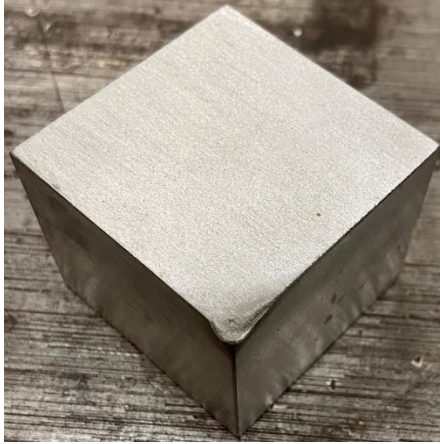
Figure 4.25 – Plinth with melted corner caused by overheating with cutting torch
