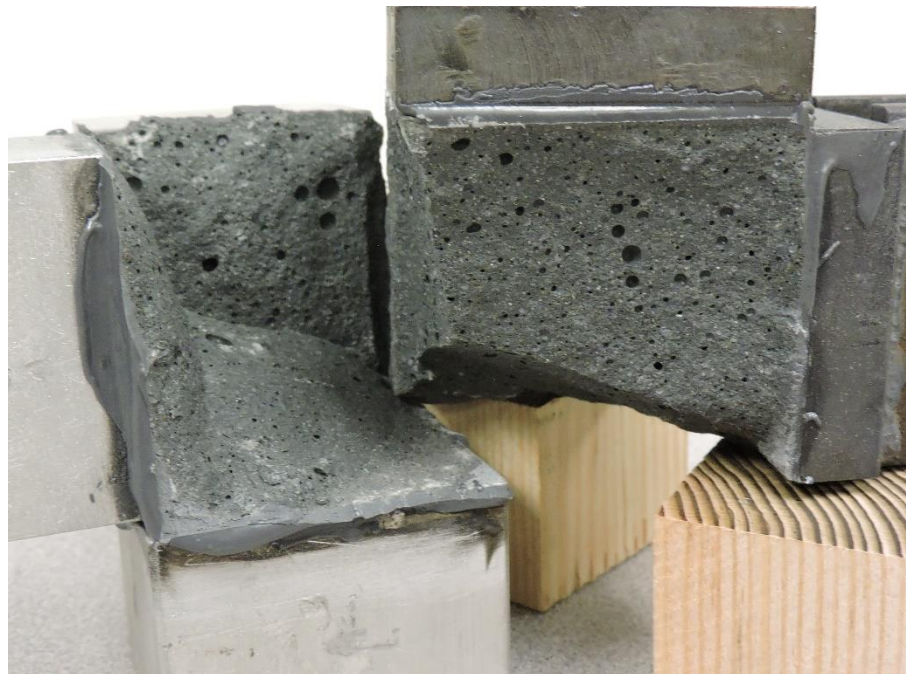
Figure 6.2 – Failed 0% cube with side where clevises stayed intact with side stresses set to 500 psi
