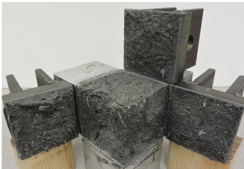
Figure 6.6 – All clevises with cone shaped concrete attached from 2% fiber specimen with side stresses set to 700 psi
