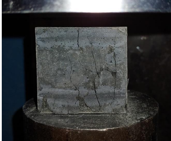
Figure 3.9 – Failed 2% cube after the uniaxial compression test
