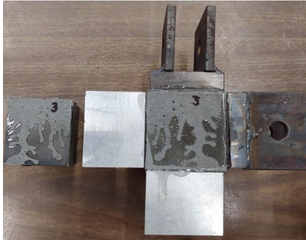
Figure 4.23 – Specimen exhibiting signs of epoxy leakage during curing
