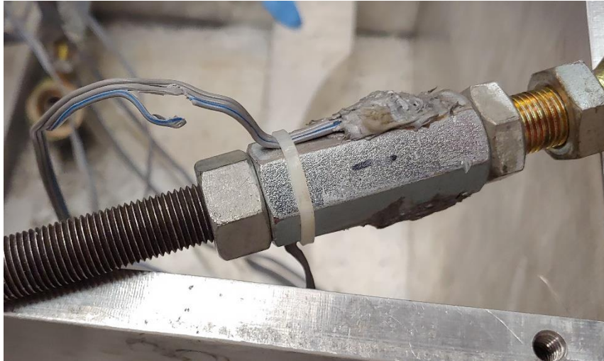
Figure 4.33 – Damage to strain gauge wire in the sigma one direction
