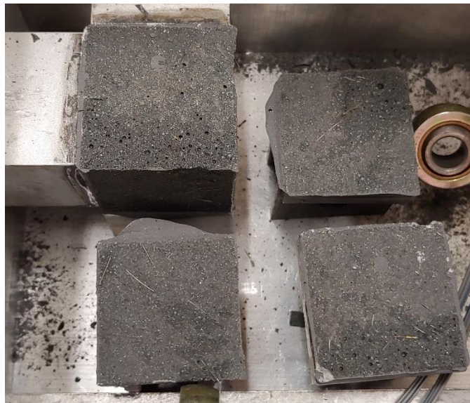
Figure 6.16 – Specimen three for 1% fibers and side stresses of 500 psi and 250 psi
