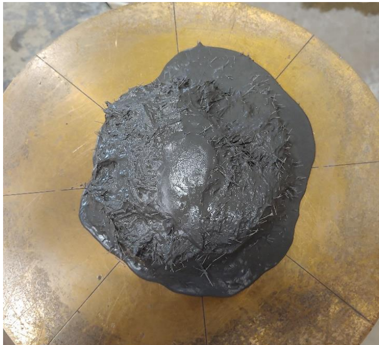
Figure 3.7 – Flow of the UHPC mix with 5% fibers
