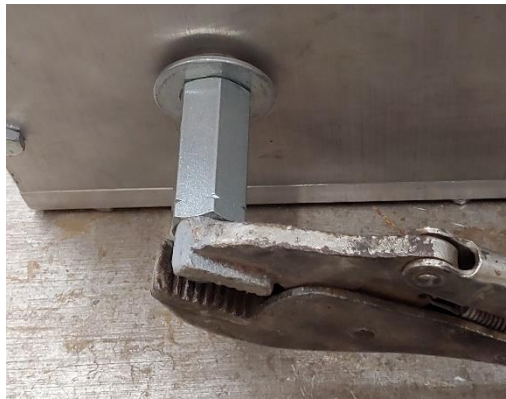
Figure 4.28 – Nut and washer setup with vice grips attached
