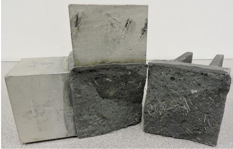
Figure 6.5 – Top clevis from failed 1% fiber specimen with side stresses of 800 psi
