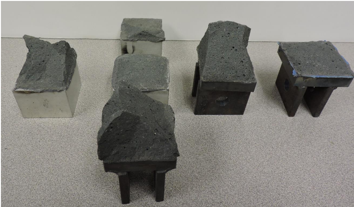
Figure 6.3 – Failed 0% cube where unusual crack patterns occurred with side stresses set to 300 psi
