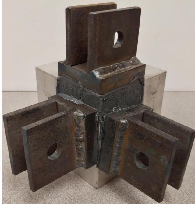
Figure 4.24 – Clevises that slid down cube due to premature removal of wood support blocks
