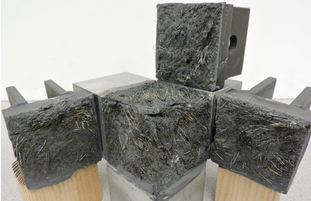
Figure 6.8 – Failure of TTT specimen with 4% fibers and side stresses of 800 psi
