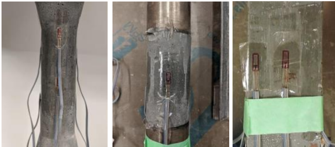
Figure 2.9 – Strain gauges applied to the dogbone (left), cylinder (middle), and prismatic (right) specimens (Lepissier, 2020)
