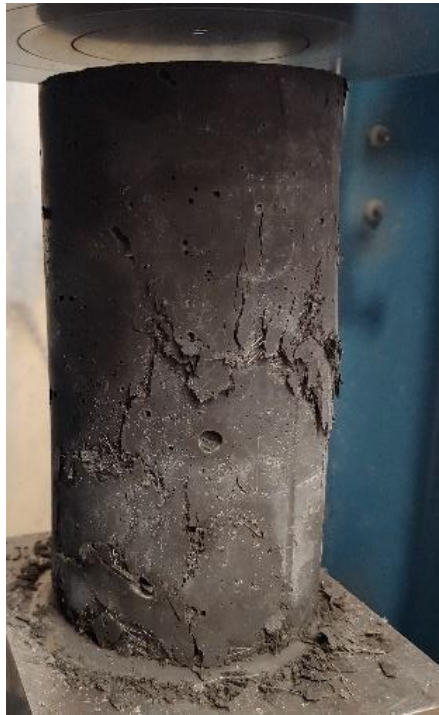
Figure 3.10 – Failed 6% cylinder after the uniaxial compression test
