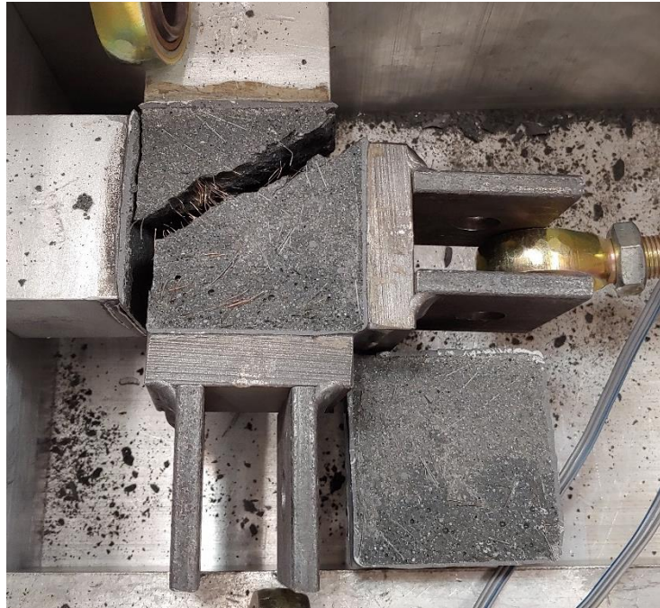
Figure 6.15 – Specimen two for 1% fibers and side stresses of 500 psi and 250 psi
