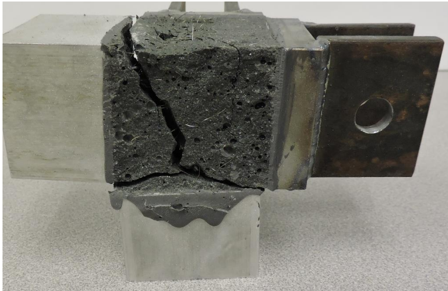
Figure 6.12 – Angled crack due to unequal side stresses with 800 psi applied through the clevis shown and 400 psi to the other clevis in 1% fiber specimen
