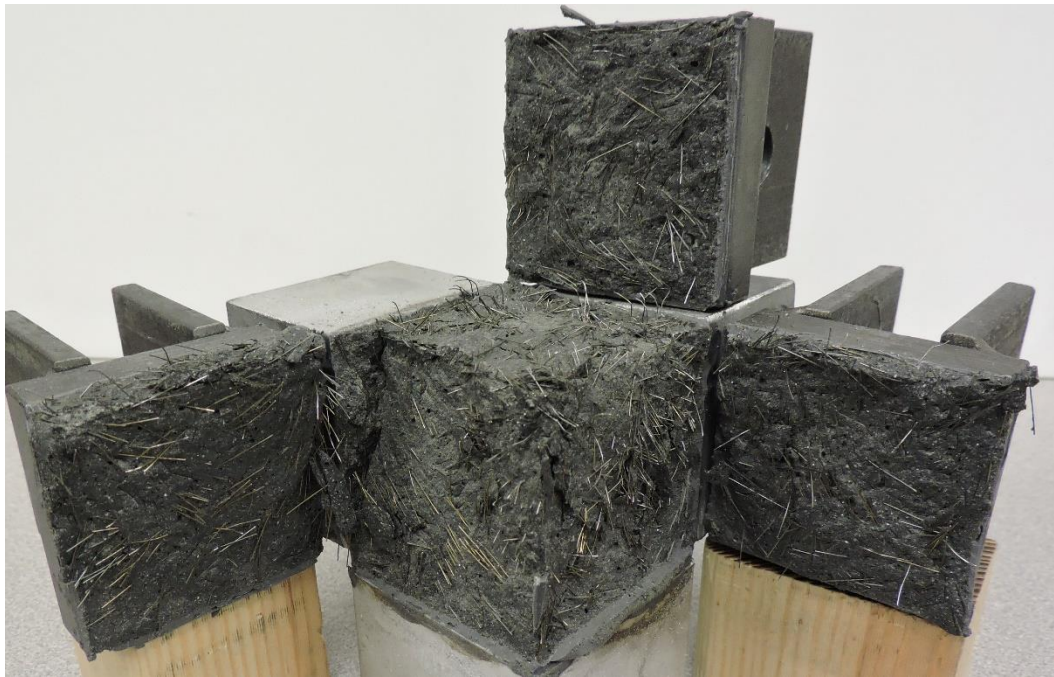
Figure 6.10 – Failed TTT specimen with 5% fibers and side stresses set to 600 psi (left side clevis) and 300 psi (right side clevis)
