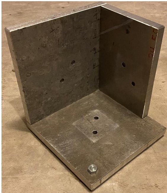
Figure 4.35 – Jig constructed for gluing two cube simultaneously
