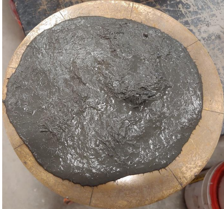
Figure 3.6 – Flow of the UHPC mix with 4% fibers
