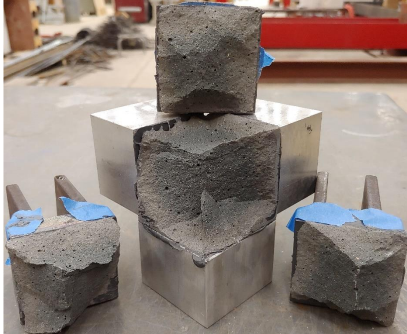
Figure 6.1 – Failed 0% cube where cube suffered substantial damage with side stresses set to 500 psi
