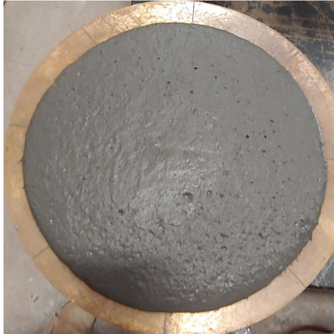
Figure 3.4 – Flow of the UHPC mix with 1% fibers
