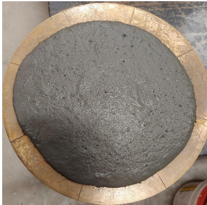
Figure 3.5 – Flow of the UHPC mix with 2% fibers
