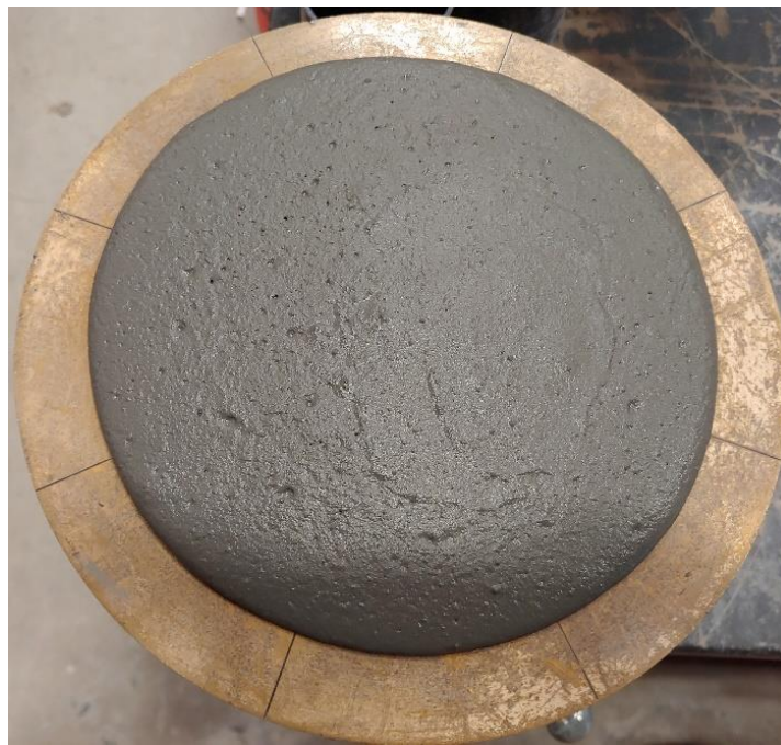
Figure 3.3 – Flow of the UHPC mix with 0% fibers
