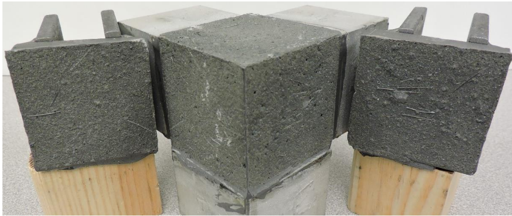
Figure 4.34 – Specimen where concrete failed at surface due to smaller clevises
