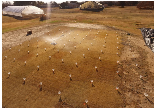
Figure 8. Catch cans arrangement to detect irrigation spray pattern uniformity at varying pressures and wind speeds.
