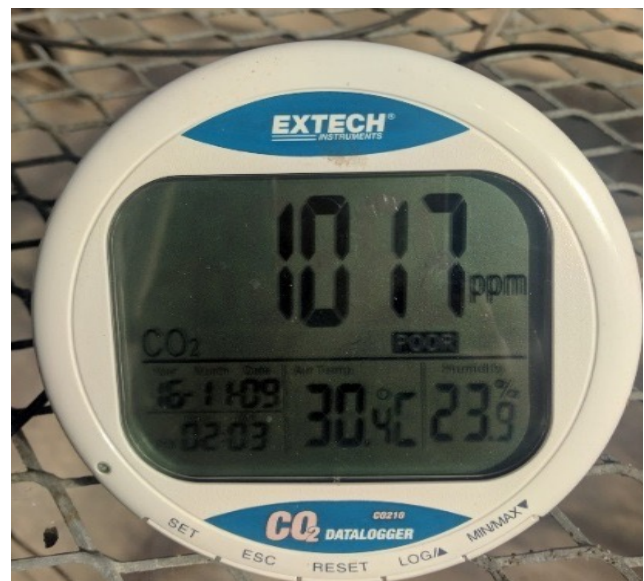
Figure 5. Extech CO 2 Monitor (FLIR Commercial Systems Inc., Nashua, NH) and data logger. It measures CO 2 , temperature and humidity and has 15,000 data log storage capacity.
