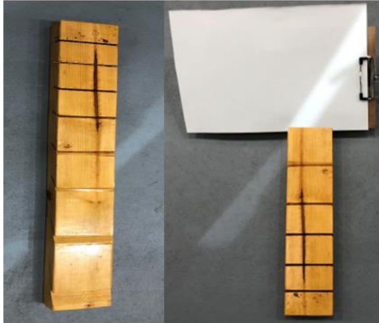
Figure 16: Impact angle experiment materials. (Left) Impact angle board with angled slot; (Right) Impact angle board with a target surface (a paper board clipped to a clipped board) placed on 40-degree angle slot. The angle of Impact board is a flat wooden board which has 9 cuts on it. Each cut on the wooden board is at different angles (10°, 20°, 30°, 40°, 50°, 60°, 70°, 80°, 90°). A wooden clip board with a white paper is placed on the angle of impact board. When the liquid blood with known volume and height is dropped on the paper, based on the angle at which the clip board is placed at the angle of stain is formed.
