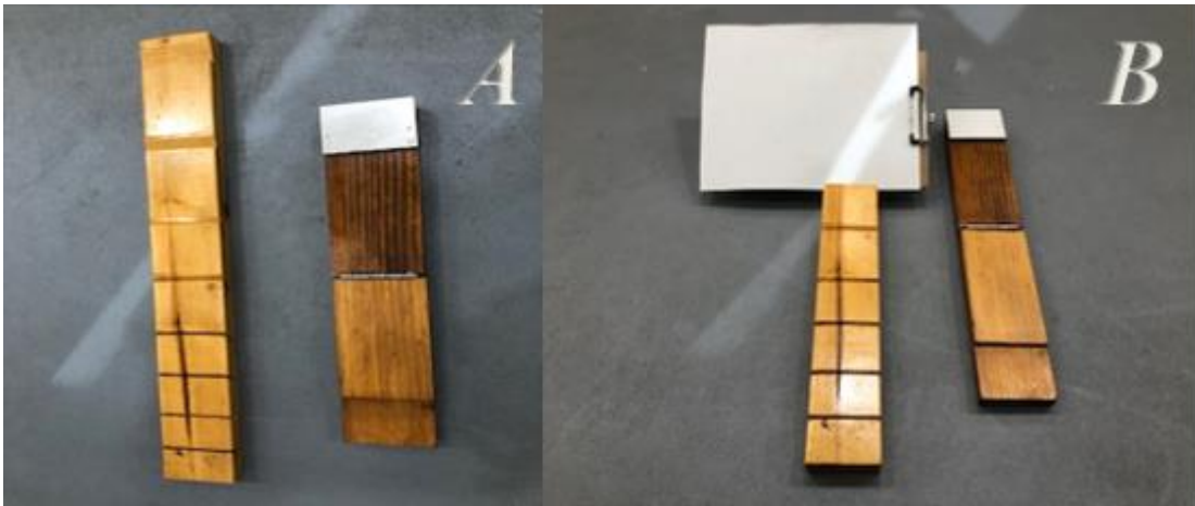
Figure 24: Photographs of a mouse trap and impact angle board (a) Mouse trap and angle board before placing a clip board (b) Mouse trap and angle board after placing a clip board at different angles.
