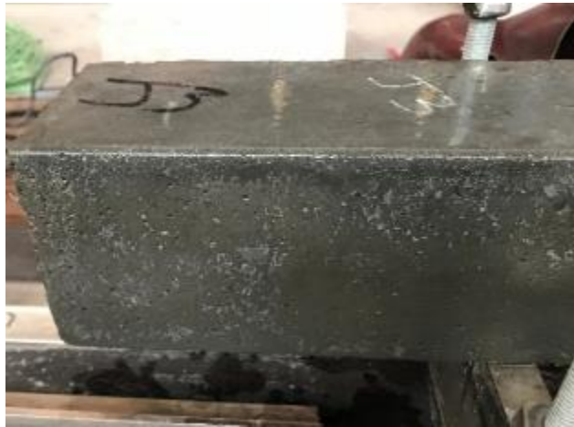
Figure 279. Deteriorated state of a J3 freeze-thaw specimen - Cycle 350
