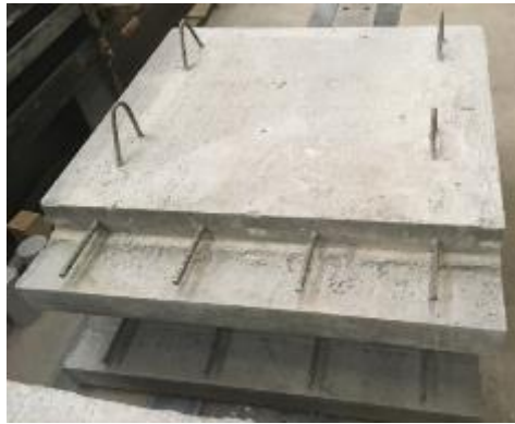
Figure 97. Completed half-depth slab specimens showing protruding rebar
