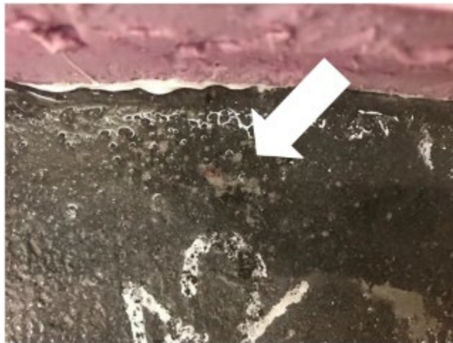
Figure 283. Visual pocketing on AA specimen - 25 cycles
