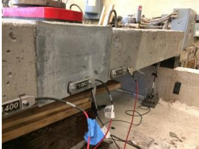
Figure 88. Placement of external strain gauges and LVDTs on the south side of the slab specimen
