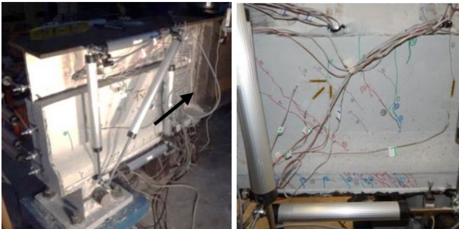
Figure 15. Repaired girder failure (Zmetra 2015)
