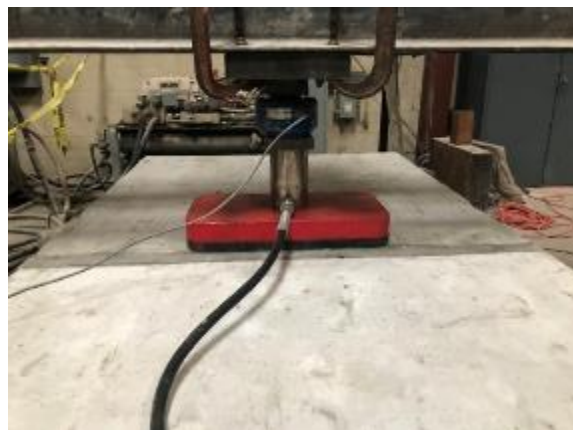
Figure 107. Test setup for slabs using the manually controlled hydraulic cylinder and pump
