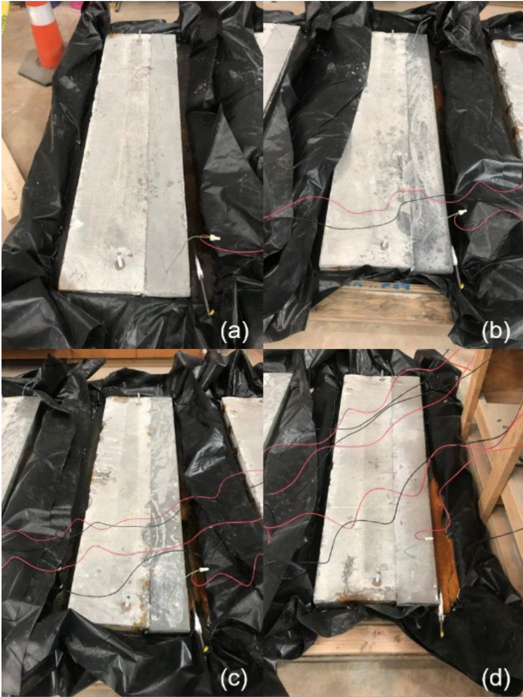
Figure 313. Week 1 update for large-scale corrosion specimens using (a) ODOT AA, (b) J3, (c) Ductal®, and (d) Phoscrete
