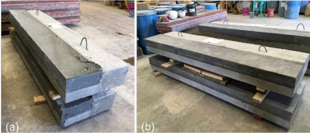
Figure 342. Completed (a) Ductal® and (b) J3 expansion joint specimens
