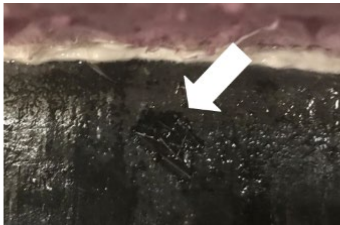
Figure 287. Visual pocketing on Ductal® specimen - 50 cycles
