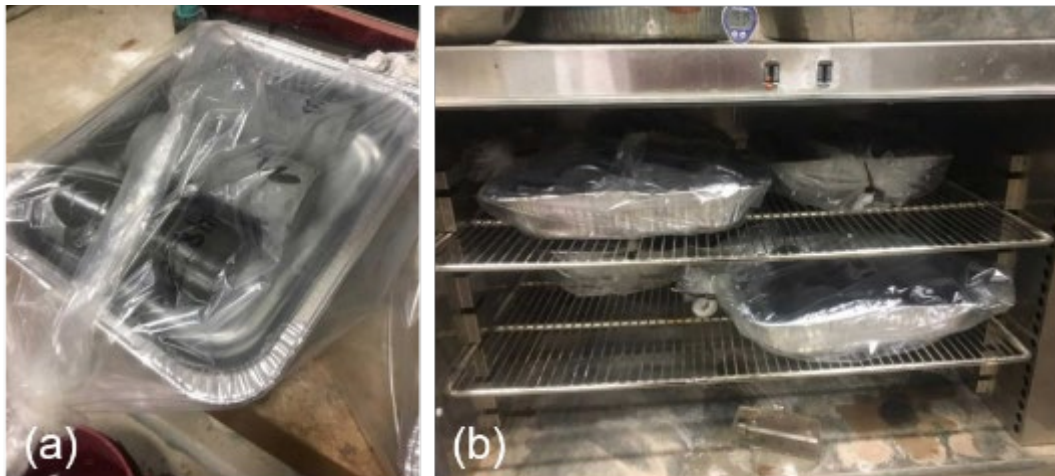
Figure 39. (a) Close-up of test specimen pan (b) overall heat curing environment of test specimens
