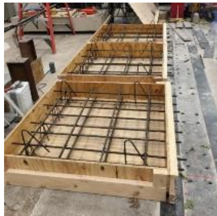
Figure 80. Formwork and reinforcement for slab specimens immediately before casting
