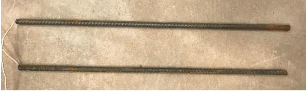
Figure 296. Steel rebar before testing - typical
