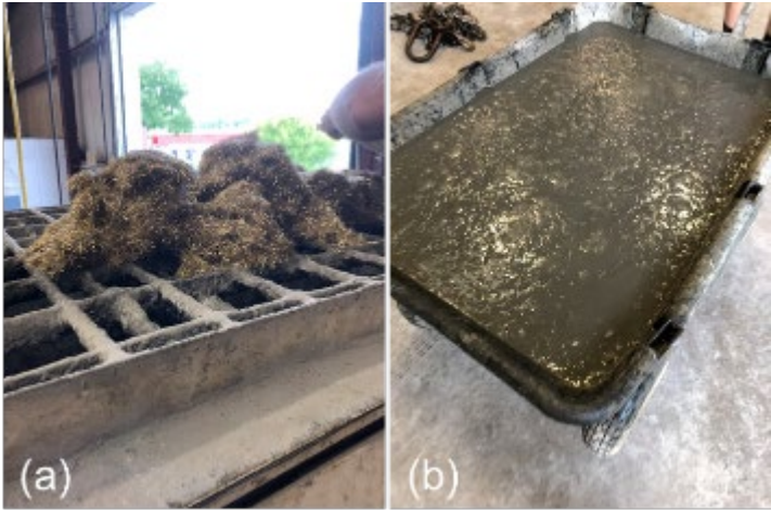
Figure 46. Revised J3 UHPC mix for composite MOR specimens (a) fiber addition and (b) transporting to formwork
