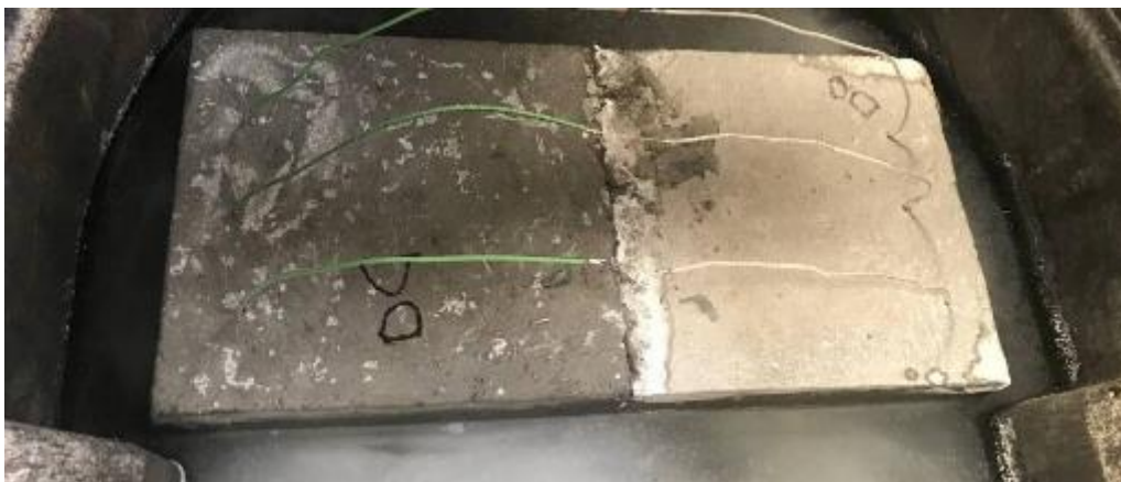
Figure 290. Initial joint corrosion in Ductal® small-scale corrosion testing specimen D0 - patching
