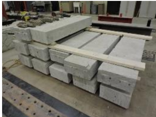
Figure 297. Large-scale corrosion joint specimens before chipping
