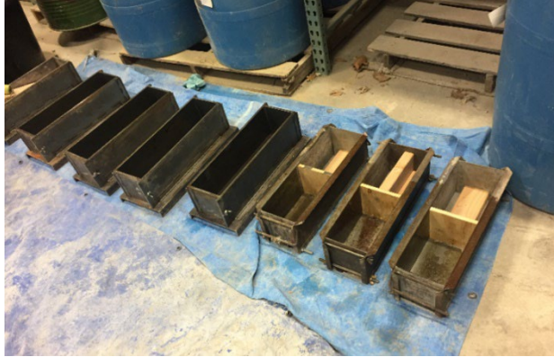
Figure 51. Formwork prepared for small-scale MOR specimens to be cast. Three half specimens for exposed aggregate finish are visible in the right of the photo
