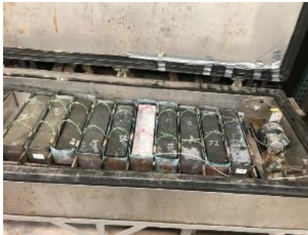
Figure 275. Freeze-thaw specimens in the testing chamber - Cycle 0
