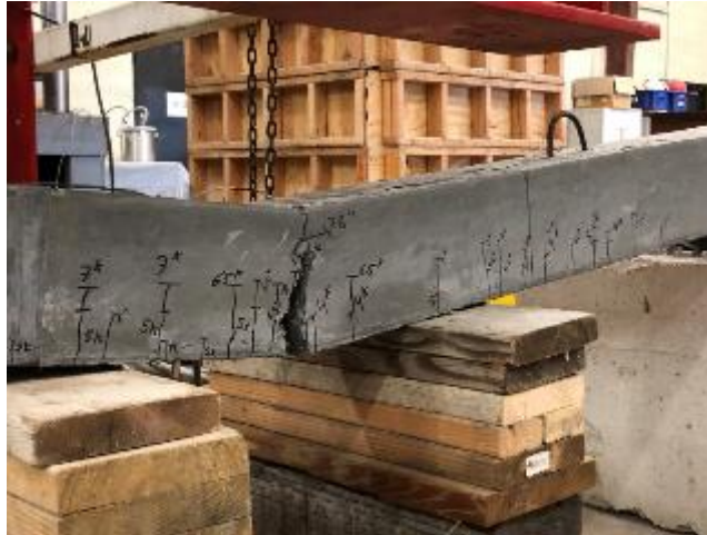
Figure 77. Crack pattern typical of SB-J5 with 2% fibers
