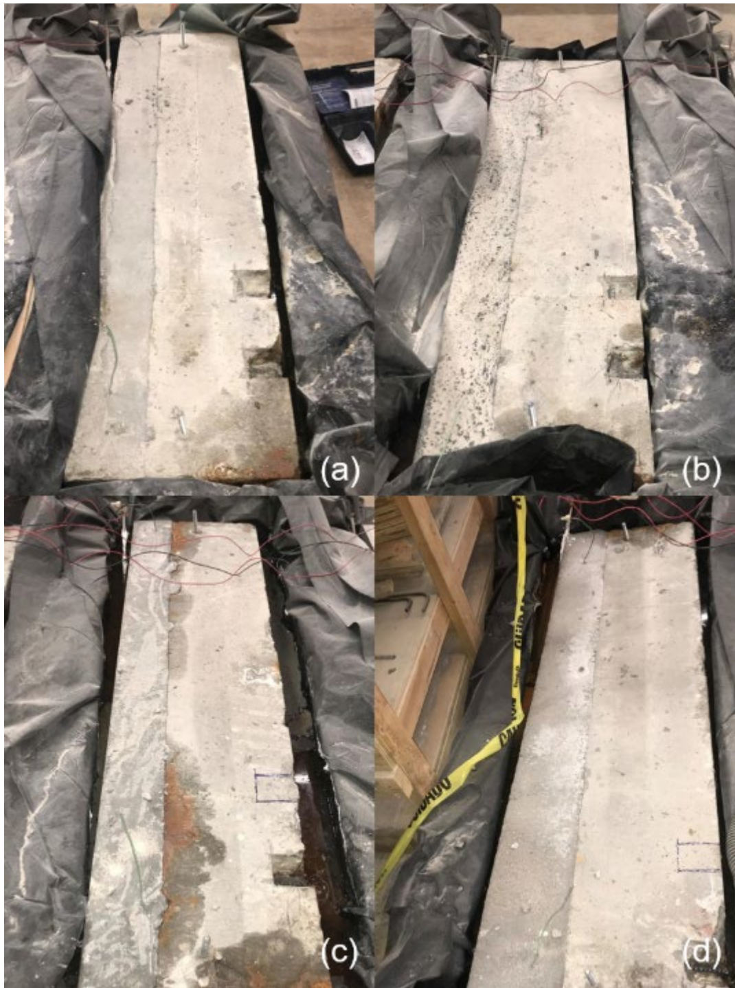
Figure 314. Week 3 update for large-scale corrosion specimens using (a) ODOT AA, (b) J3 (c) Ductal®, and (d) Phoscrete
