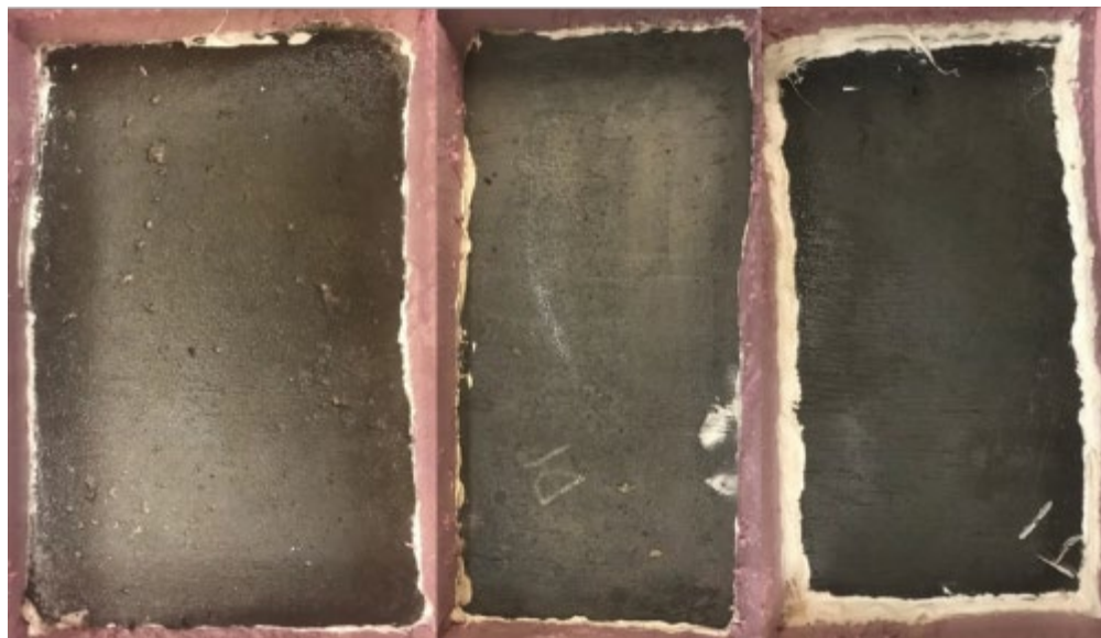
Figure 285. Visual examination of scaling specimens at 50 Days for ODOT AA (left), Ductal® (middle), and J3 (right)
