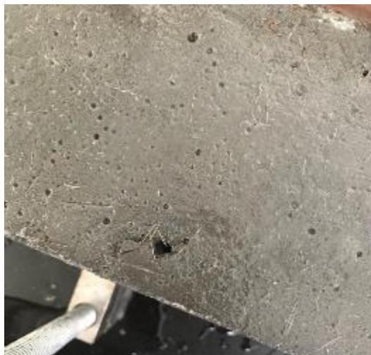
Figure 280. Hole formed on the side of Ductal® freeze-thaw specimen - Cycle 315
