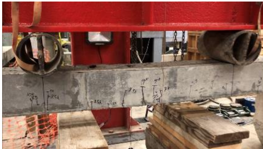
Figure 76. Crack pattern for test SB-D5-2
