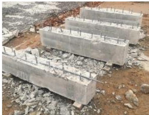
Figure 298. Large-scale corrosion joint specimens after chipping
