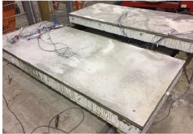
Figure 8. Final experimental panel with UHPC overlay used by Khayat et al. (2018)
