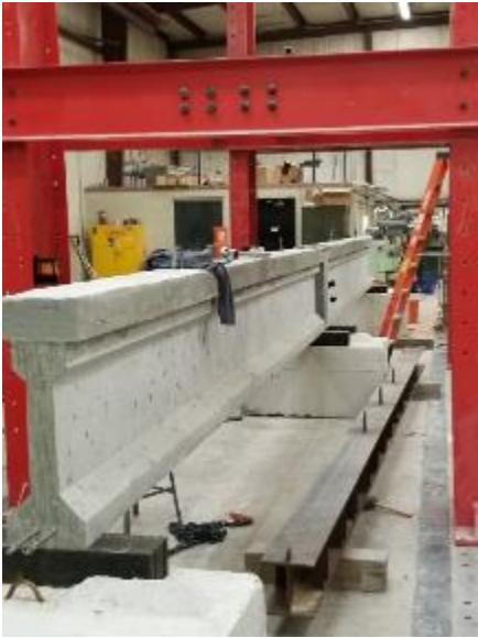
Figure 195. Continuity joint specimen in place for testing
