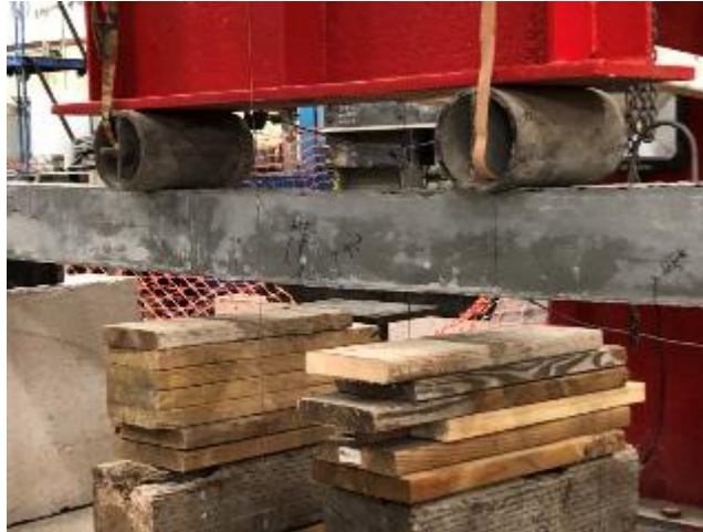
Figure 75. Crack pattern for test SB-D5-1
