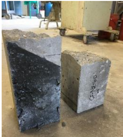
Figure 57. Example of failure pattern for one of the 60° joint specimens
