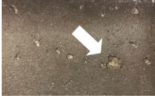
Figure 286. Progression of visual pocketing on AA specimen - 50 cycles
