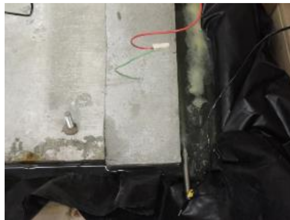
Figure 302. White film in water of Phoscrete large-scale corrosion specimen
