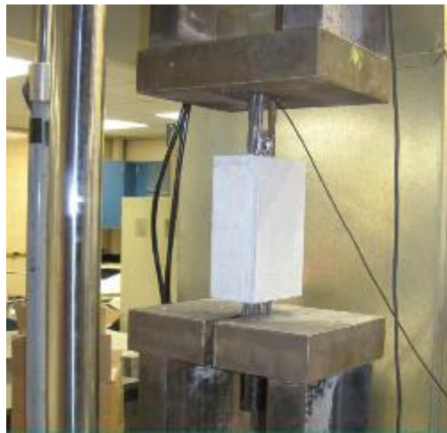
Figure 28. FHWA prestressing strand-UHPC bond test specimen in load frame (Graybeal 2014)
