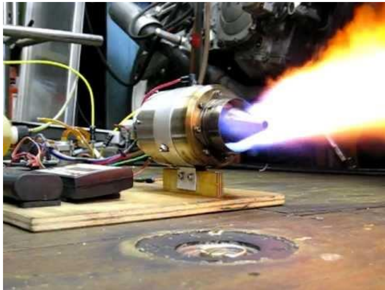
Figure 11: Combustion with Rich Fuel Mixture [3]
