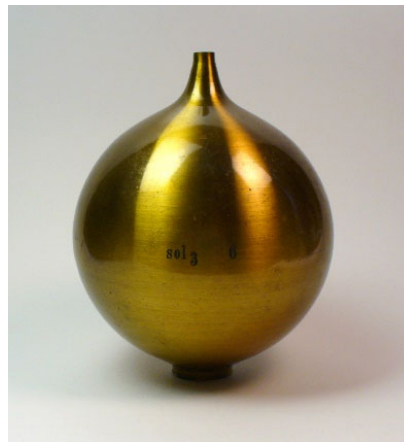
Figure 3: Helmholtz resonator, top inserted in-ear, bottom open to a sound source [15]
