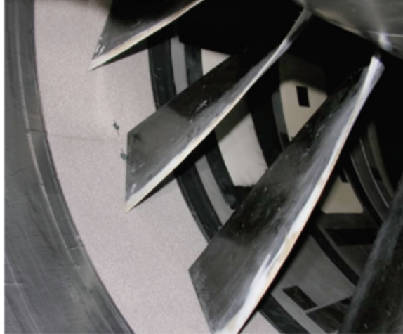
Figure 12: Foam metal liner (developed by Sutliff and Jones) installed in an engine test stand [49]
