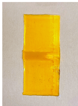
b) The 4D printed LCE hinge at undeformed, neutral state
