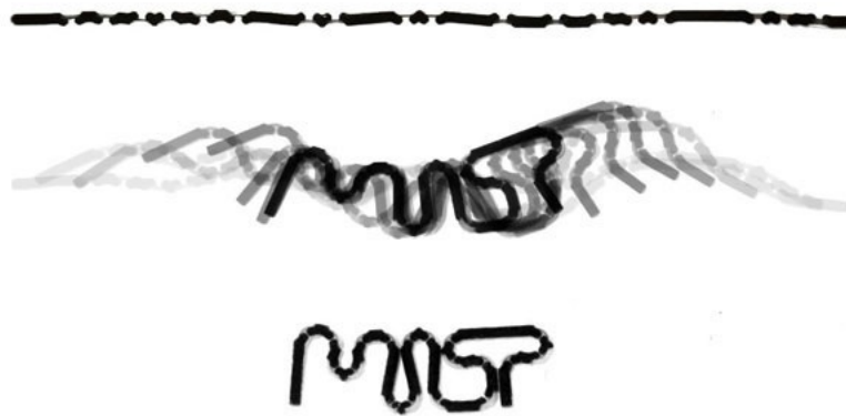
Figure 3: Example of a 1D to 2D deformation of a 4D printed material [3]
