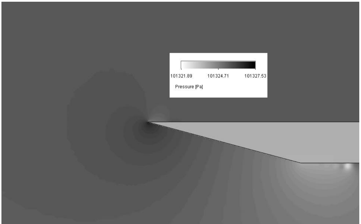
Figure 16: Pressure increase at leading edge of the plate
