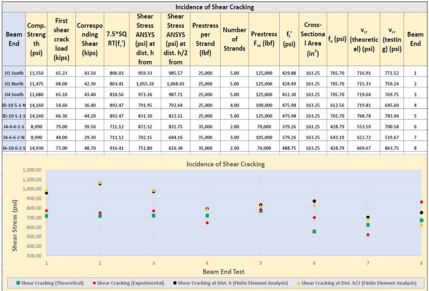
Figure 3.17. Shear Stresses Compared with Results of FEA at Distances h and h/2 from Support
