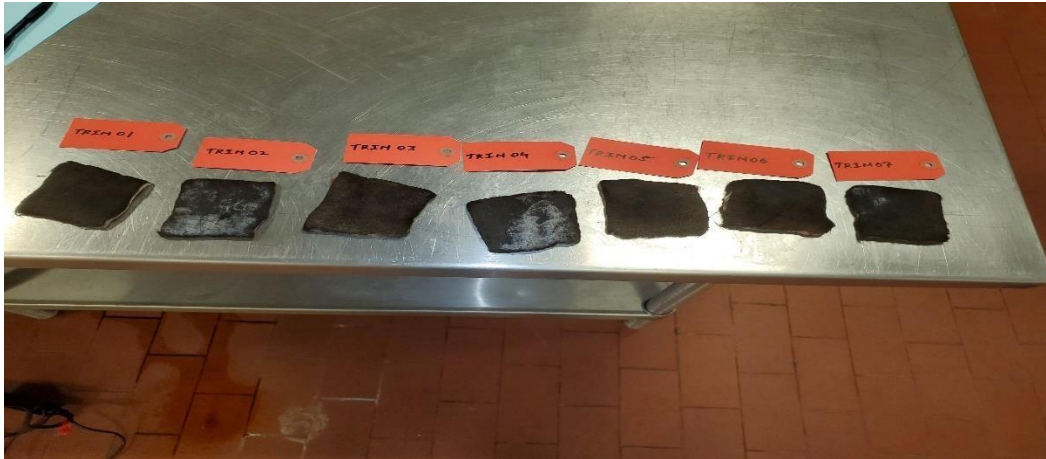
Rawhide squares after trimming the hair with Trimmer
