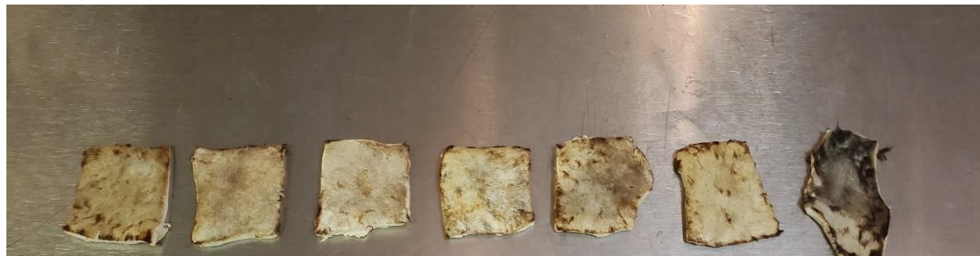
Raw hides after dehairing with sodium hydroxide and hydrogen peroxide
