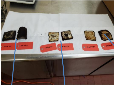
Picture 2: Hide squares after scorching and scraping.
