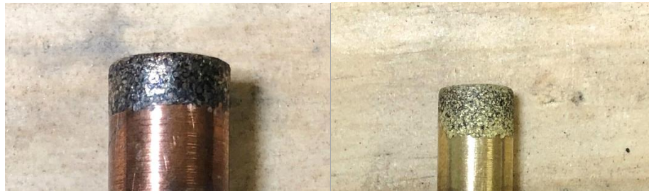
Figure 23: Copper electrode (left) has much more slag than the brass electrode (right)
