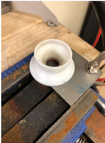
Figure 15: E-Drill locator piece and test piece secured in vice
