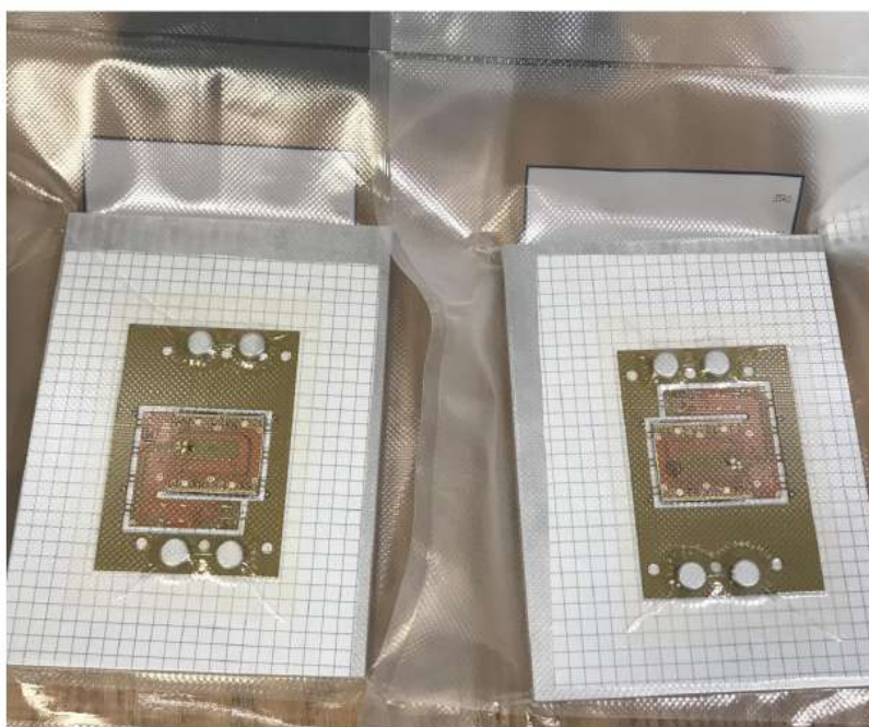
Figure III.3: The rice paper assembly method uses a vacuum sealed bag to apply even pressure to the flex cable and sensor hybrid. A rice paper piece that has been cut to the correct dimensions and infused with adhesive is sandwiched between the two. The grid paper shown is a thick, clean room safe paper that is cut to align the sensor hybrid in place.
