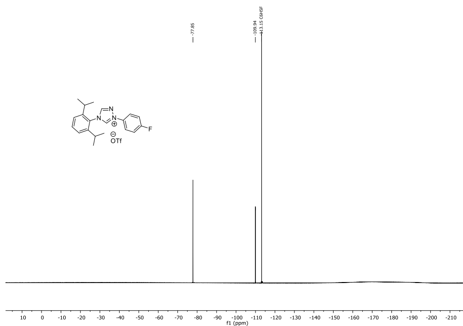
Figure D107: 19 F NMR spectrum of 4-(2,6-diisopropylphenyl)-1-(4-fluorophenyl)-4H-1,2,4-triazol-1-ium trifluoromethanesulfonate ( [8e]OTf ) (376 MHz, DMSO- d 6 , 298 K, referenced to fluorobenzene).
