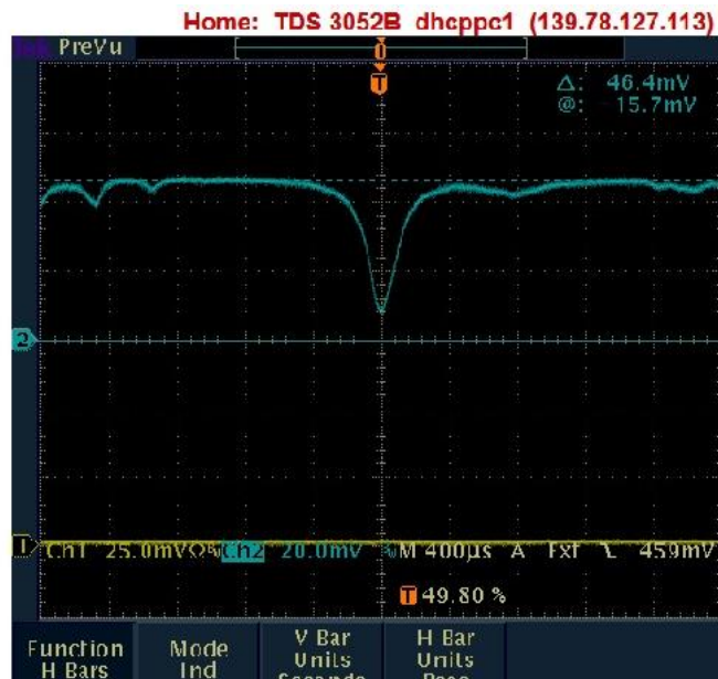
Figure 1.3. Symmetric Lorentzian dip. This WGM has \Delta\nu = 20.7 MHz, Q = 9.1 \times 10^6 , and M = 0.83 .
