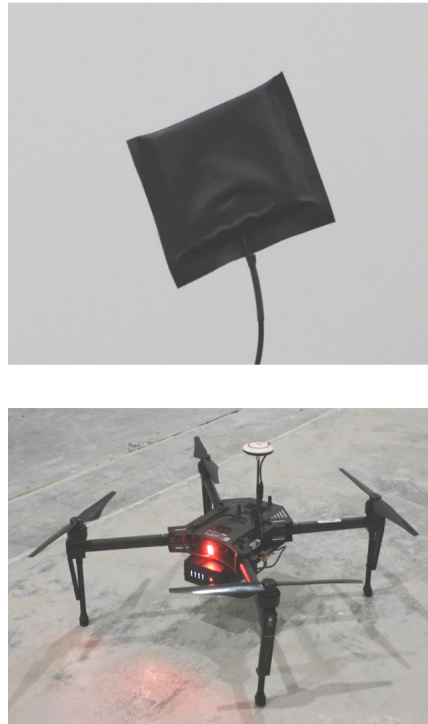
Figure 30: Octave antenna and IRIS+ quadcopter
