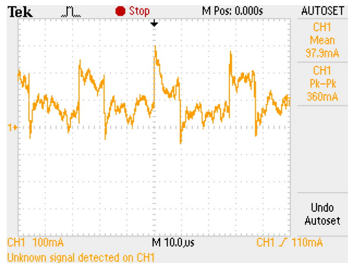
Figure 3.14, Current Measurement through SEPIC's for Second Inductor with 63% Duty Cycle
