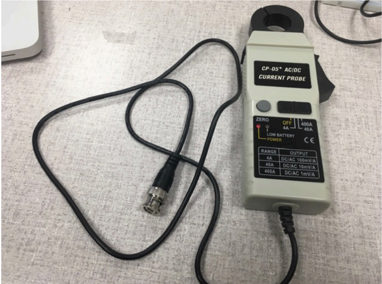
Figure 3.6, Current Probe used for Measuring Inductor Current
