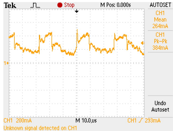
Figure 3.13, Current Measurement through SEPIC's for First Inductor with 63% Duty Cycle
