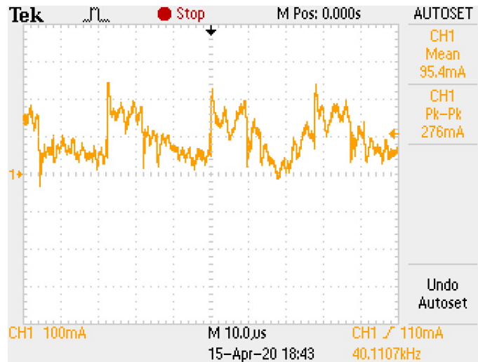
Figure 3.12, Current measurement through SEPIC's for Second Inductor at 52% Duty Cycle
