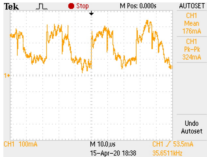
Figure 3.11, Current Measurement through SEPIC's for First Inductor at 52% Duty Cycle
