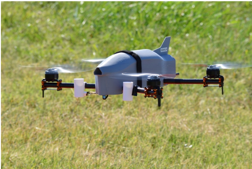
Figure 3. Most recent (2019) version of rotary-wing OU CopterSonde, courtesy Brian Greene. The most apparent differences between the design of this most recent version and the version of the OU CopterSonde in Figure 2 is the more rectangular shaped, boxed body of the aircraft and more defined nose cone for drawing in air in the most recent version of the OU CopterSonde.
