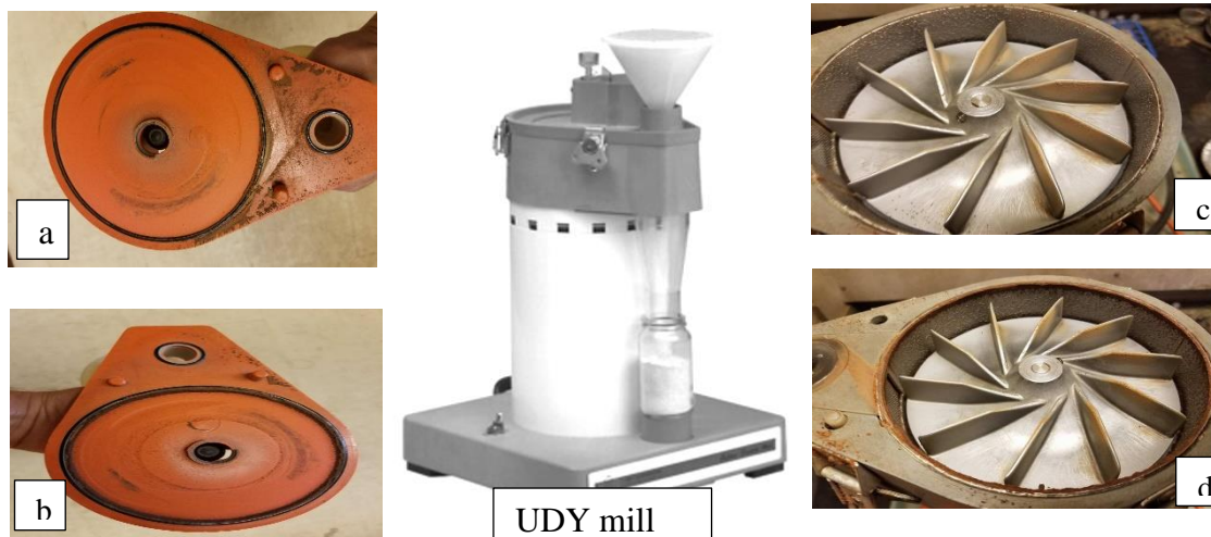
Fig. 21. Different parts of UDY mill; Mill cover after grinding press cake (b) and grape seed (a), grinding ring and chamber after grinding press cake (c) and grape seed (d)
