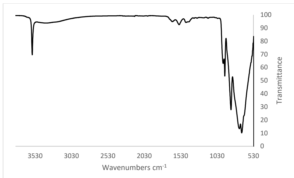
Figure 3.1. Infrared Spectrum of Y(MoO_4)(OH) \cdot H_2O
