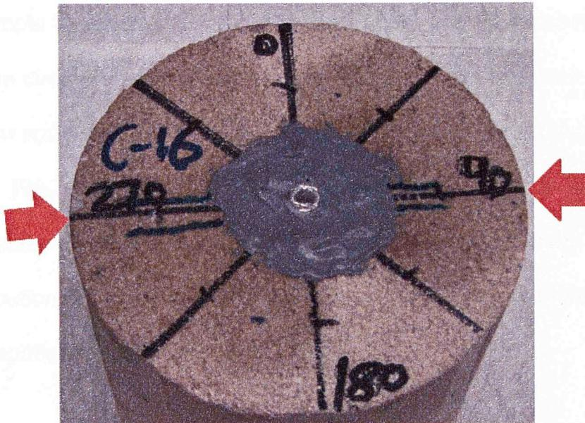
**Fig. 4.19** - Surface view of sample C16 showing a fracture development in the direction of the stress applied (red arrows). The fracture is enclosed by the dark blue lines.
