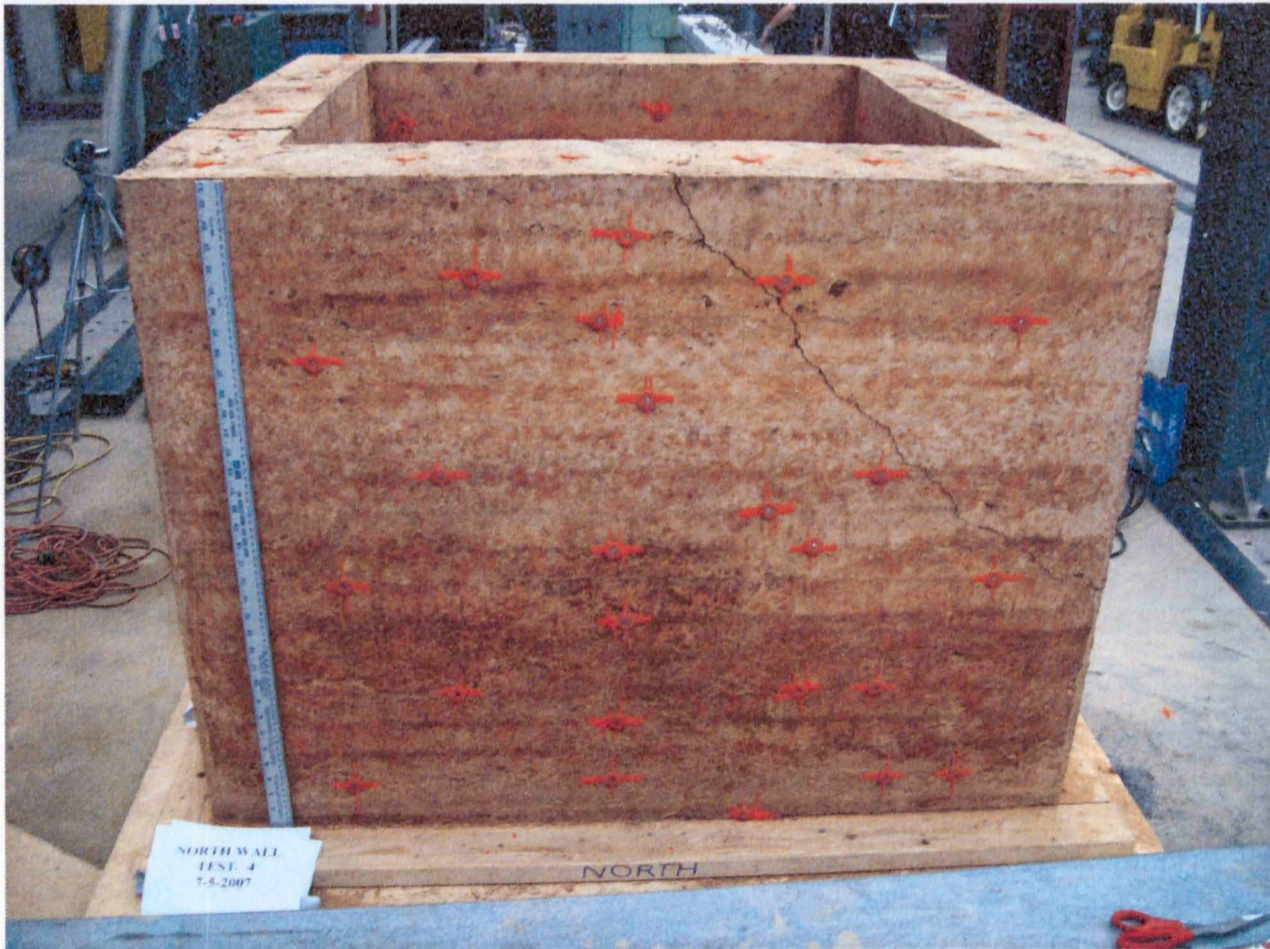
Figure 3.49: Test 4 view of diagonal crack along north wall after test
