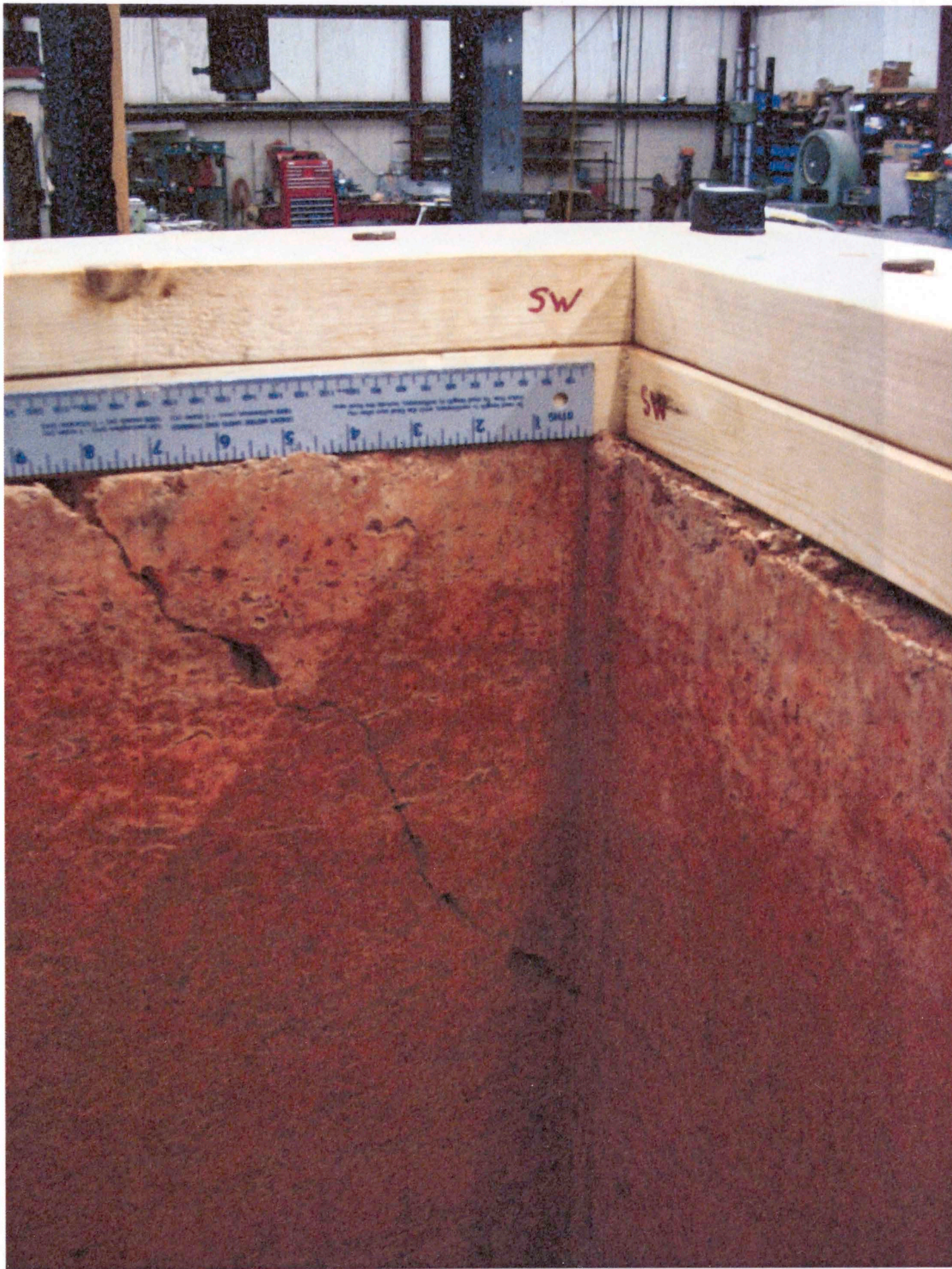
Figure 3.39: Test 3 measurement of diagonal crack at interior of SW corner
