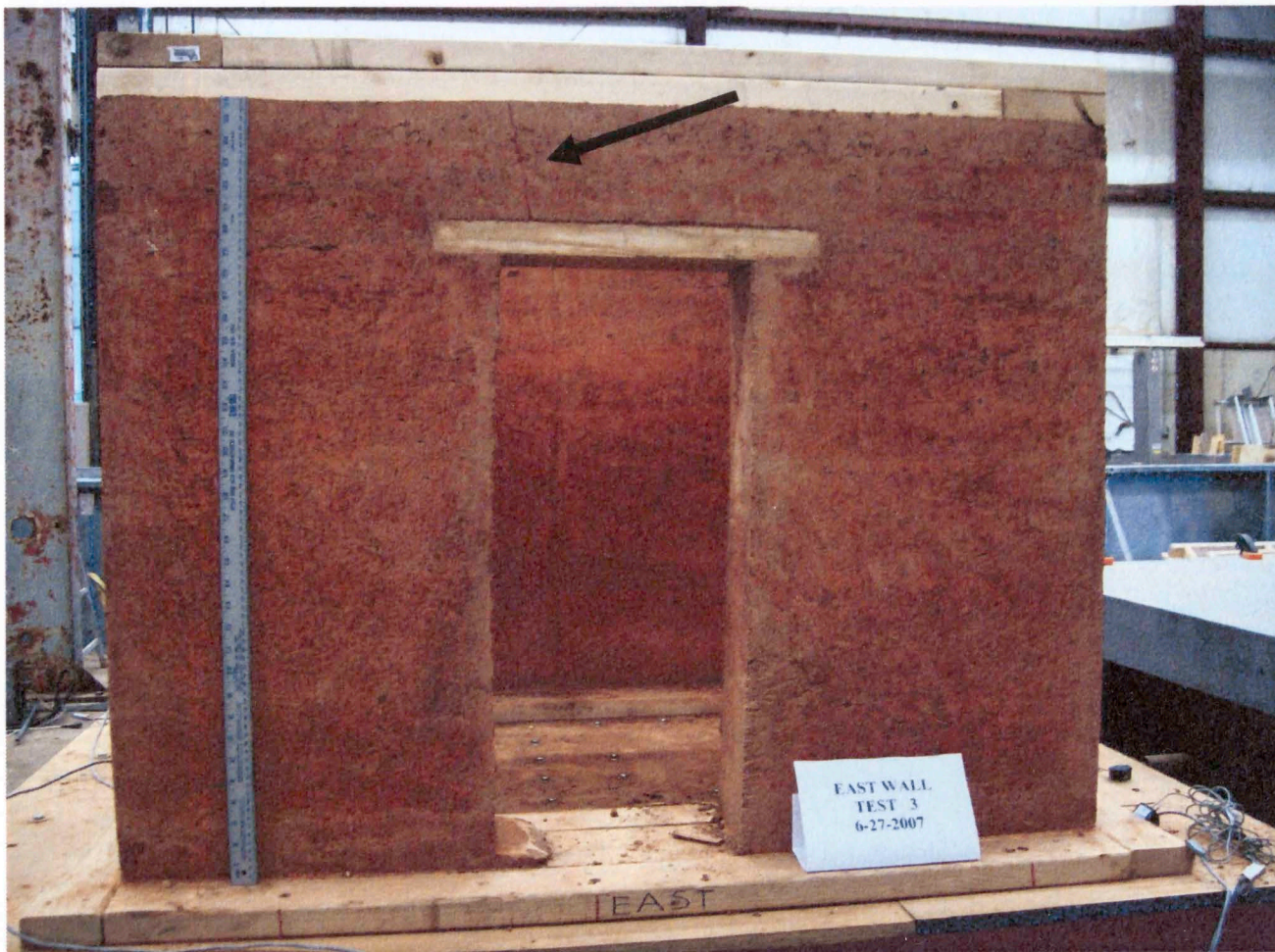
Figure 3.27: Test 3 view of east wall before test, note crack above door opening
