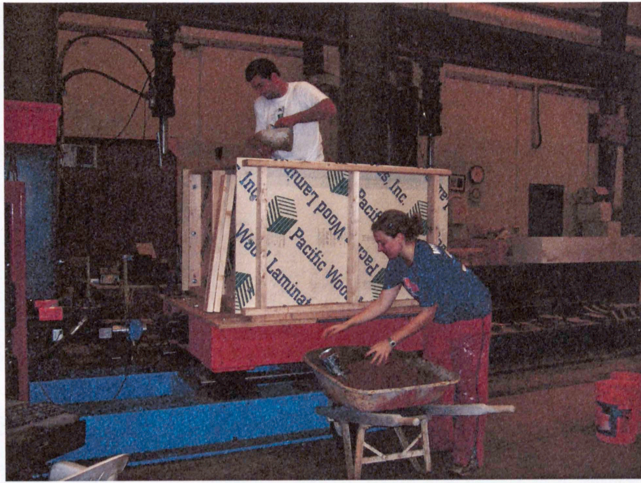
Figure 2.18: Placement of soil into formwork
