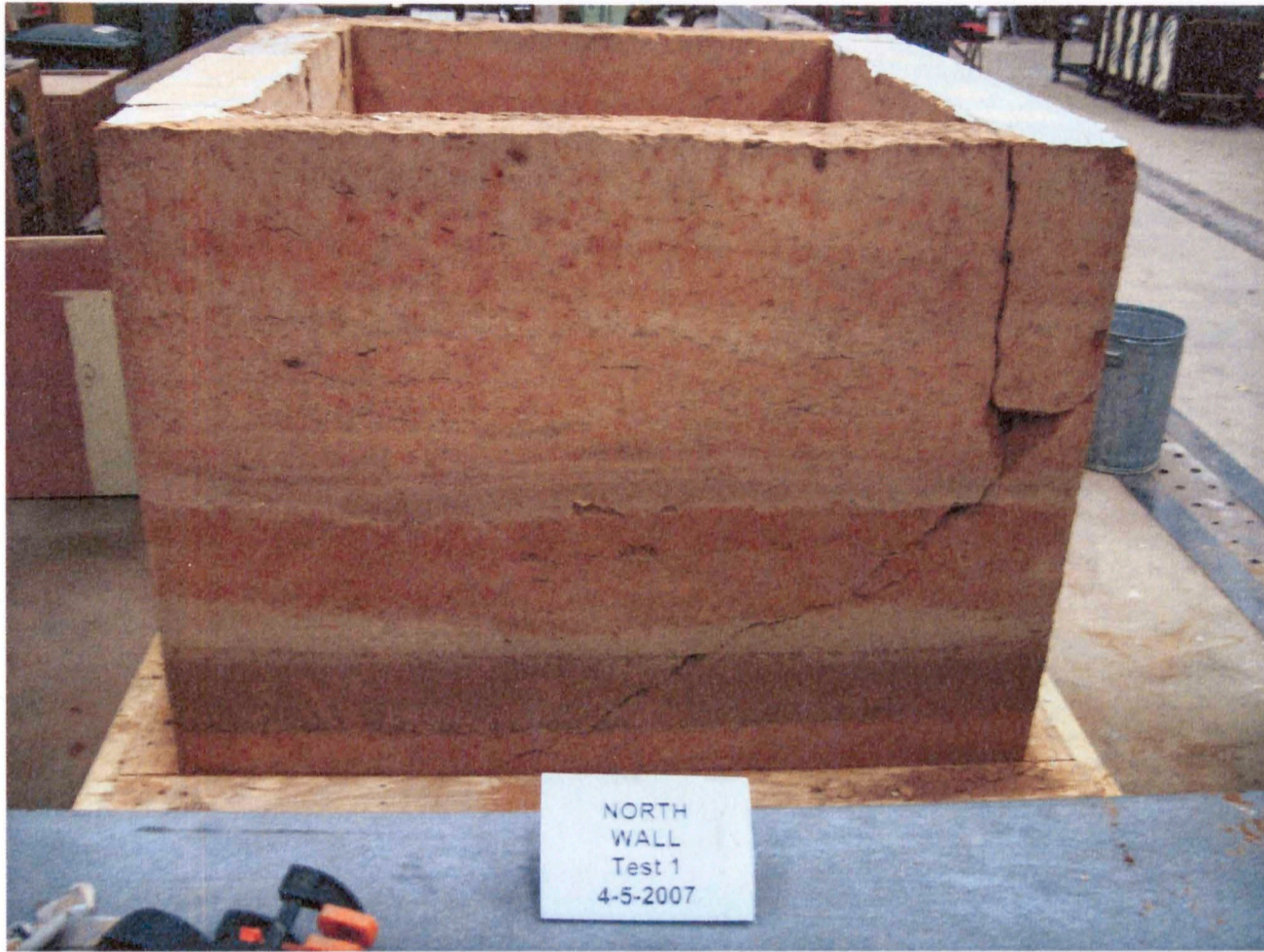
Figure 3.9: Test 1 diagonal crack on exterior north wall
