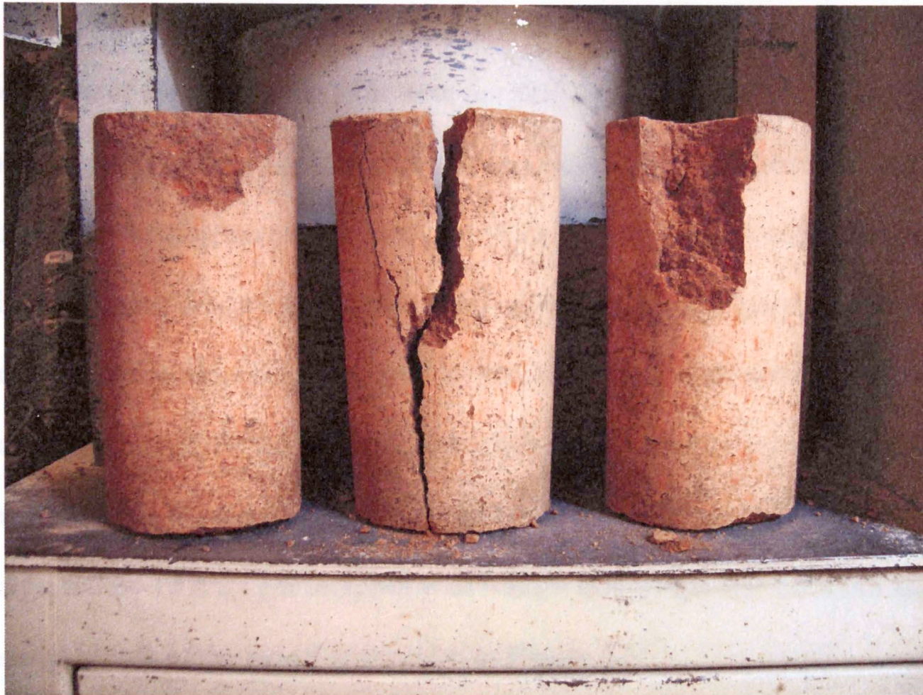
Figure 2.2: Typical failures of test cylinders
