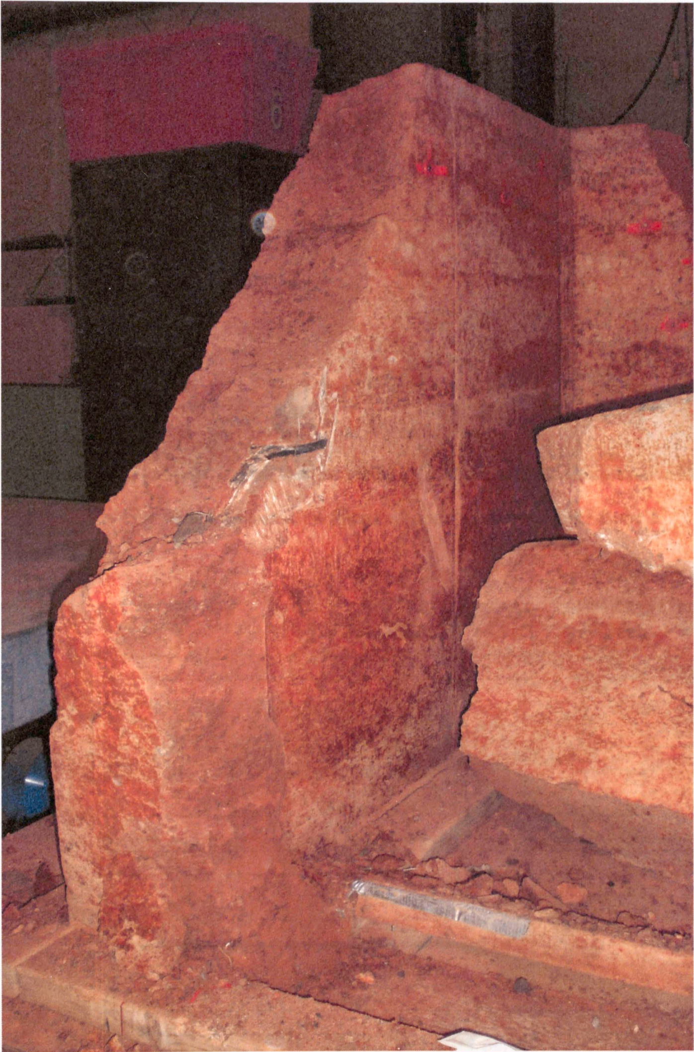
Figure 3.52: Test 4 view of exposed failure planes at north and west walls during demolition
