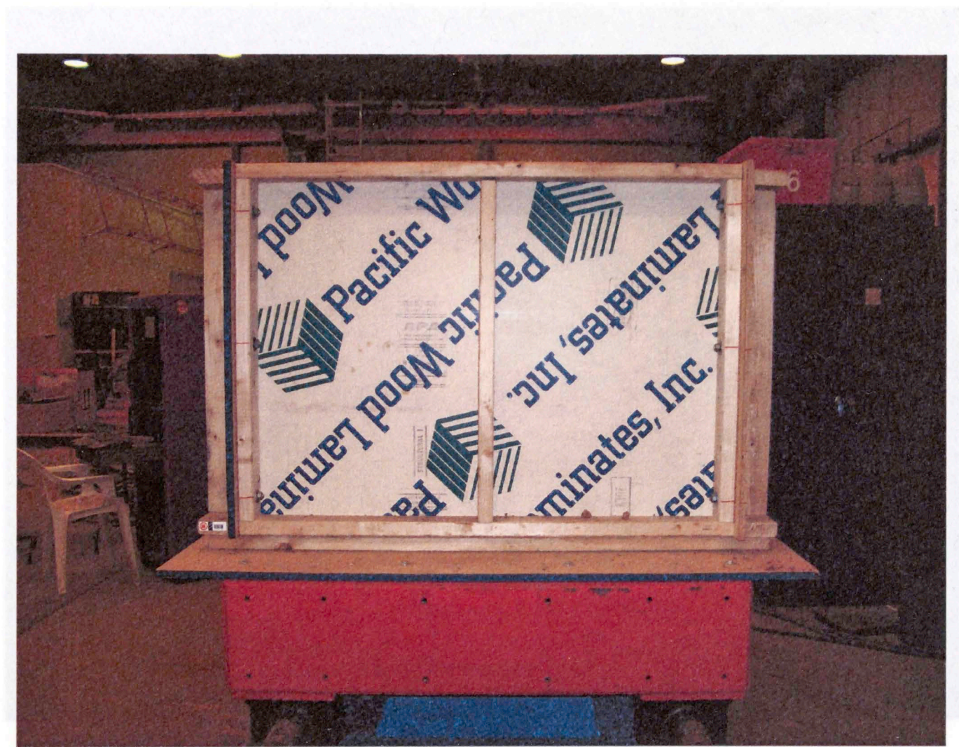
Figure 2.9: Picture of shorter outer wall formwork
