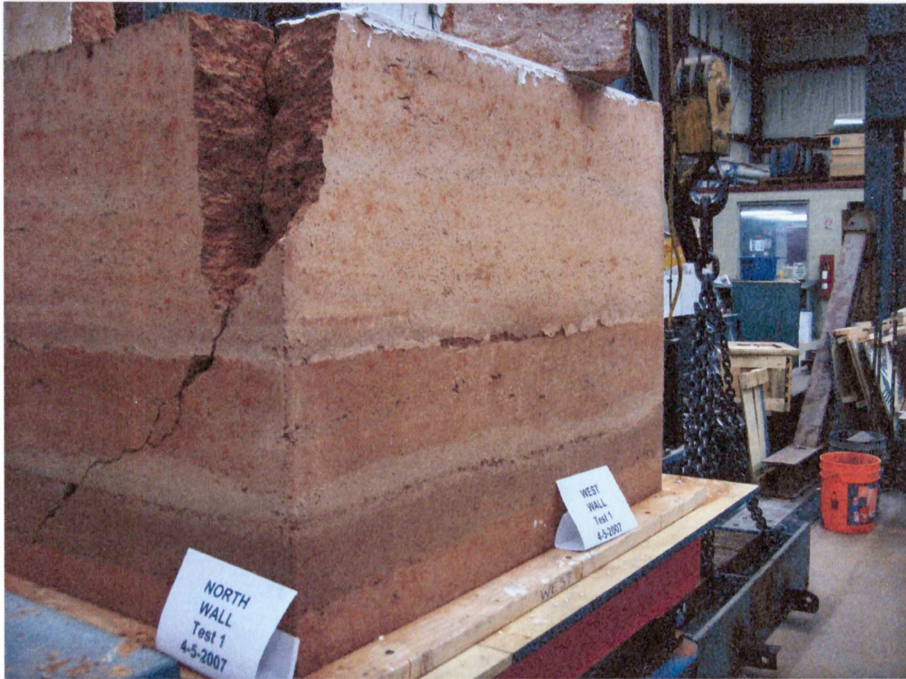
Figure 3.7: Test 1 elevation view of cracked northwest corner after test
