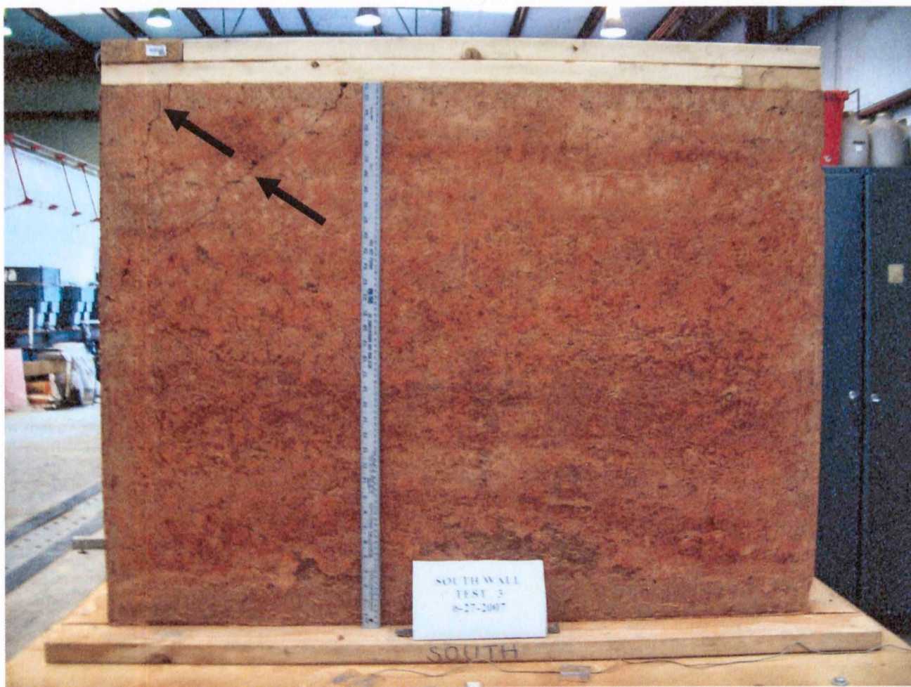
Figure 3.37: Test 3 view of south wall after test. Arrows point to fractures
