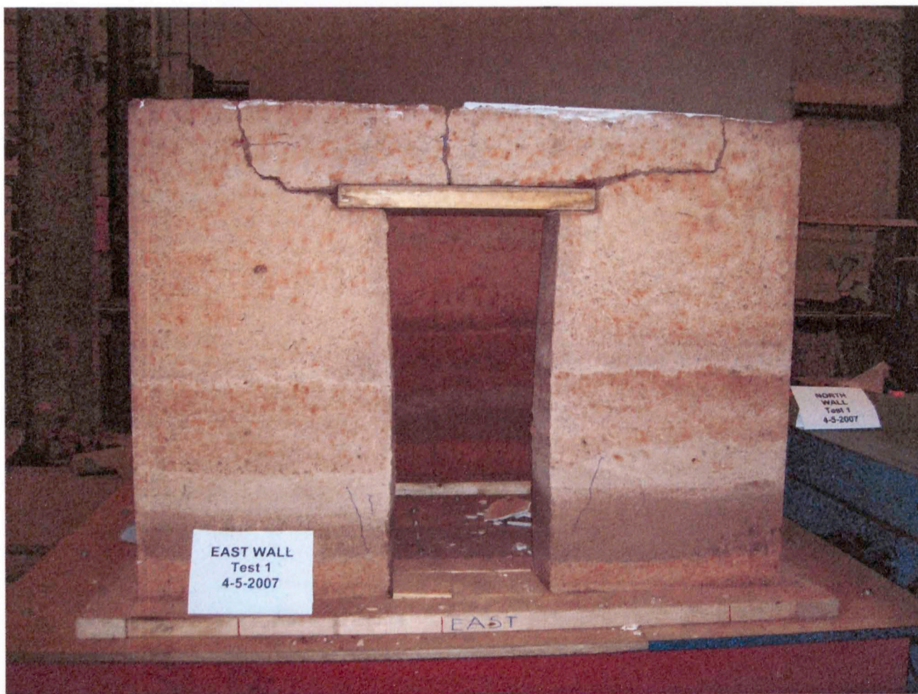
Figure 3.2: Test 1 cracks above lintel in east wall after test
