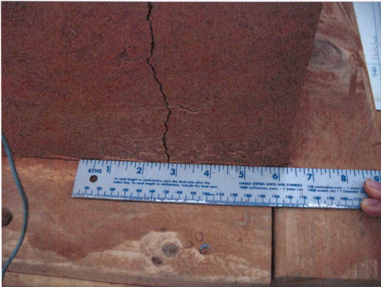
Figure 3.34: Test 3 width of fractured section at SW corner along base of west wall
