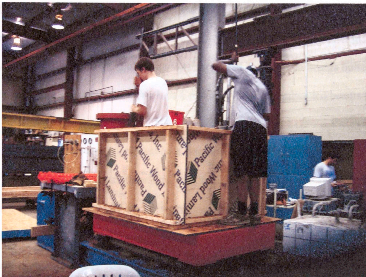
Figure 2.20: Compaction of soil with steel tampers
