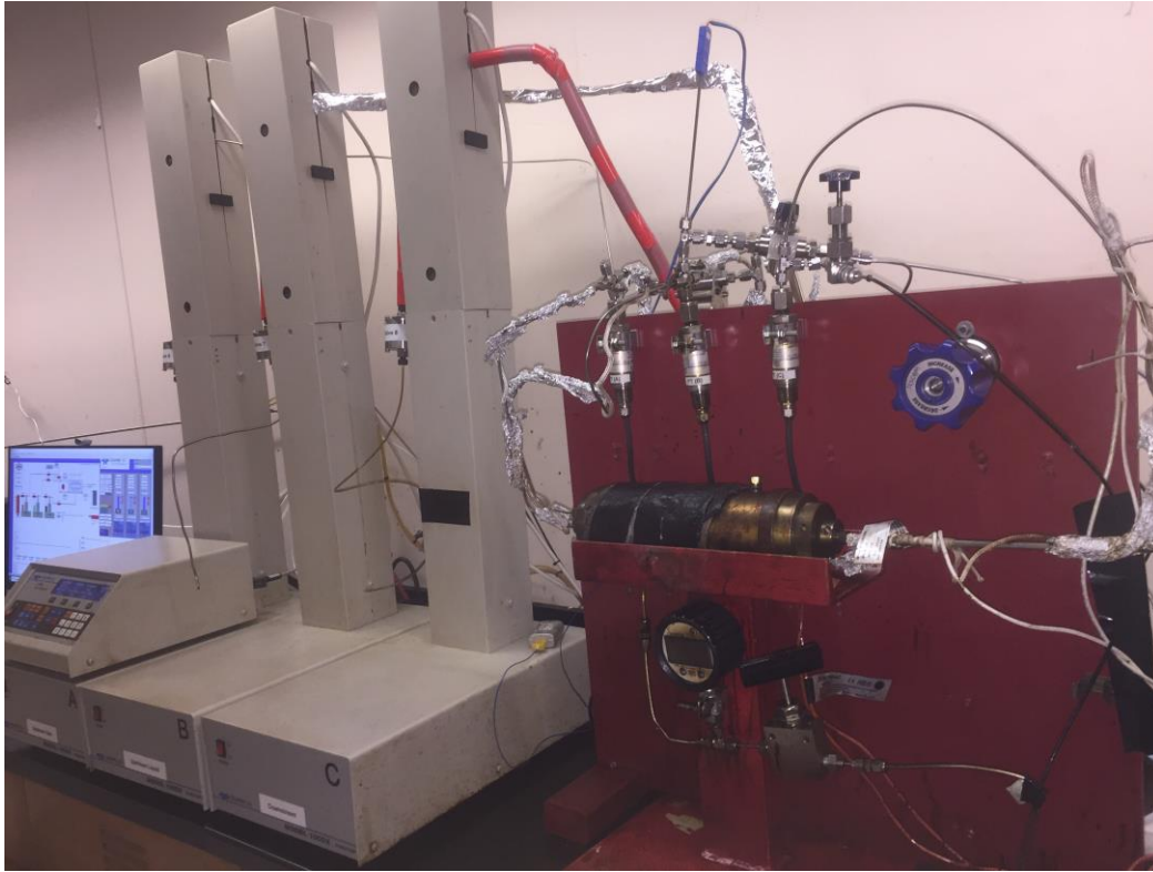
Figure 3.8: Picture of the apparatus used for the co-injection of oil and gas.
