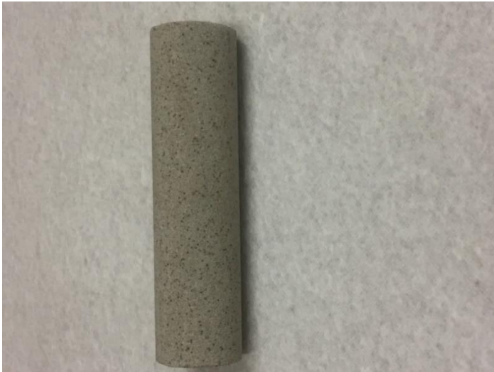
Figure 4.1. Picture of the Berea sandstone core plug used for the experiments.
