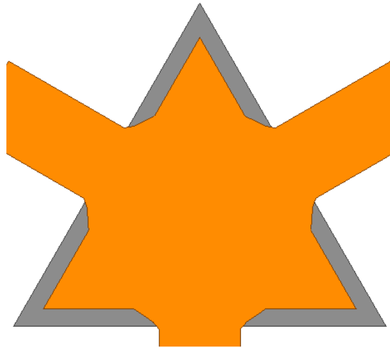
Figure 3.6: Closeup of the center conductor of the junction used in all simulation models and the tapering that prevents local maximums of RF magnetic energy.
