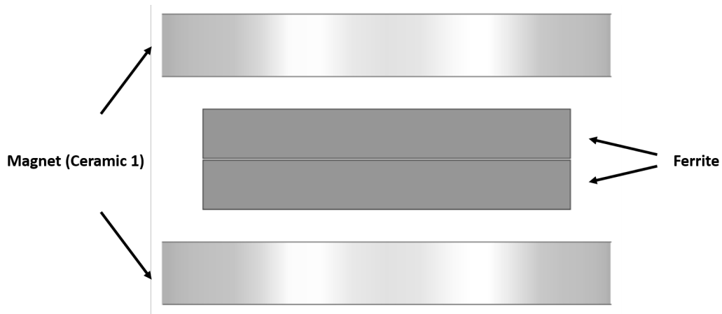
Figure 2.5: Side view of a Maxwell model, depicting ferrites being biased via permanent magnets.
