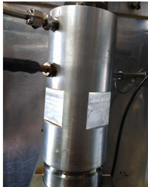
Figure 4.4: Assembled MFS and test housing for experimental set up. A) The rotor was slid over the shaft and secured against the stator ring. B) A closing cap with hydraulic ports was closed the housing.
