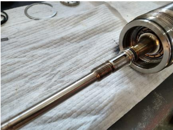
Figure 4.3: Test housing assembly used for the experimental set up. A) Drive shaft inside the testing cylinder. B) Stator subassembly showing back springs used to provide the closing force on the seal.
