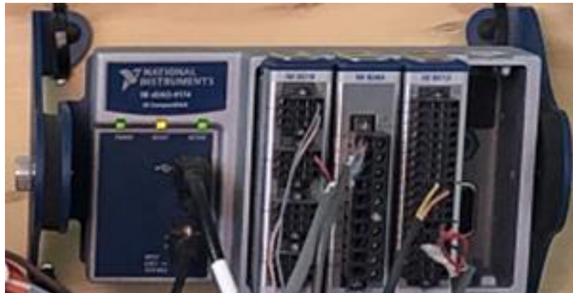
Figure 4.12: National Instruments Data Acquisition Modules as installed in the experimental set up. Each module receives signals from sensors to control the different sub systems
