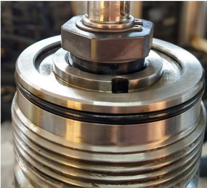
Figure 4.4: Assembled MFS and test housing for experimental set up. A) The rotor was slid over the shaft and secured against the stator ring. B) A closing cap with hydraulic ports was closed the housing.
