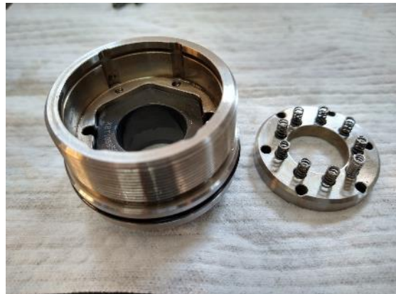
Figure 4.3: Test housing assembly used for the experimental set up. A) Drive shaft inside the testing cylinder. B) Stator subassembly showing back springs used to provide the closing force on the seal.
