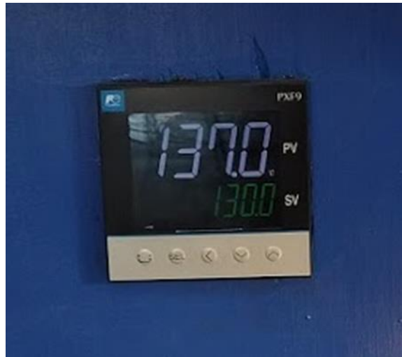
Figure 4.11: PID controller model PXF9 provided by Omega. This controller is used to drive the heating system of the experimental set up.
