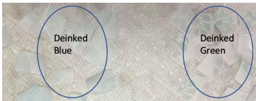
Figure 9: Deinked with (4.12g) NPEO 10 and (4.12g) PEI at pH 12 after 4 hour agitation.
