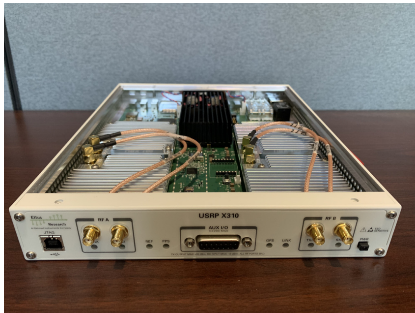
Figure 3.1: X310 pictured with top cover removed to show daughter cards installed.
