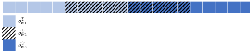
Figure 5.13: The sliding averaging window used to generate the estimates of \widehat{\sigma}_{\mathbf{W}}^2 . Here a frame length of 20 is shown with a window length of 10.
