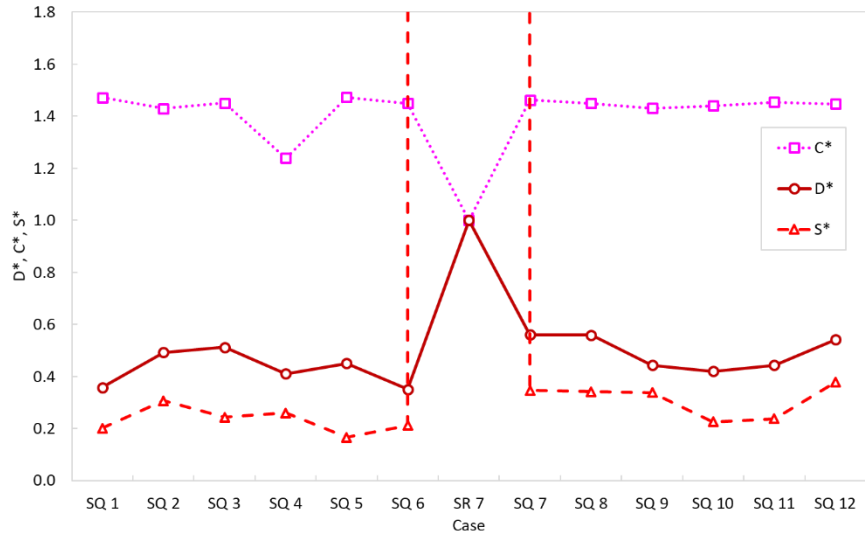
Figure 3.15: Output displacement ( D^* ) and power spectral ( S^* ) transmissibility and normalized wave speed ( C^* ) for the resonator sequence variation cases.
