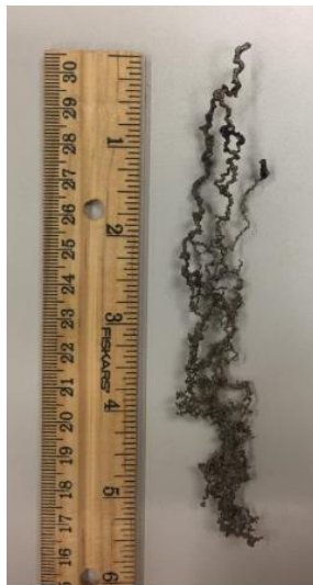
(a) Core 2: oil-saturated, 1,100 psi, 0.27 PV bt
