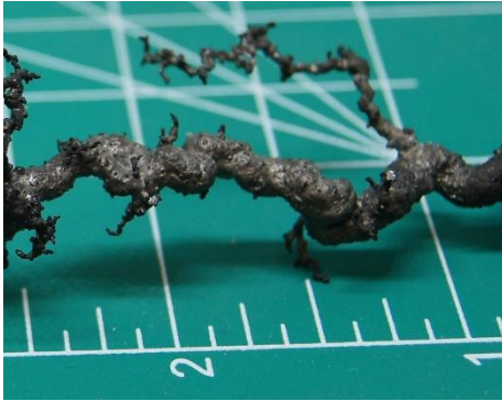
Figure 6.39: Wormhole of water-saturated core
