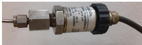
Figure 6.9: Pressure transducers used
