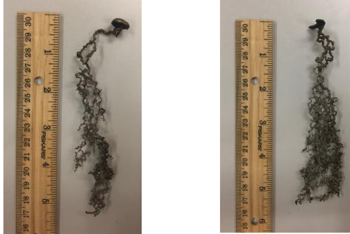
(a) Core 42: oil-saturated, 1,100 psi, 0.29 PV bt (b) Core 45: oil-saturation, 3,000 psi, 0.24 PV bt
