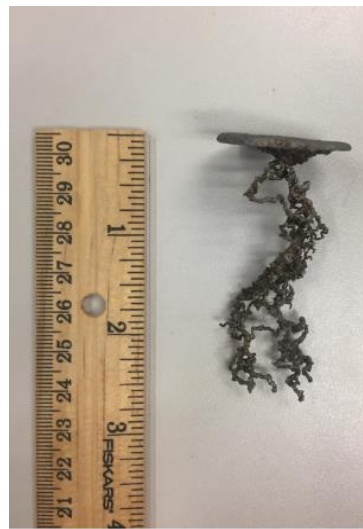
(b) Core 27: oil-saturated, 3,000 psi, 0.57 PV bt
