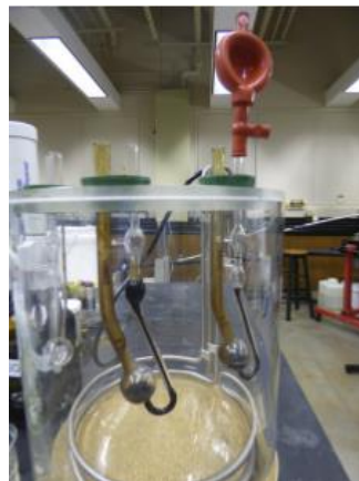
Figure 4.1: Measuring viscosity using Cannon capillary viscometer (Scarborough 2016)
