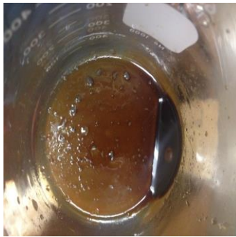
Figure 4.20: A picture of the effluent emulsion taken directly after acid injection into LS-4, a crude-saturated core, where acid was injected into the core at 3.5 cm 3 /min with the outlet pressure kept constant at 1,200 psi (Scarborough 2016)
