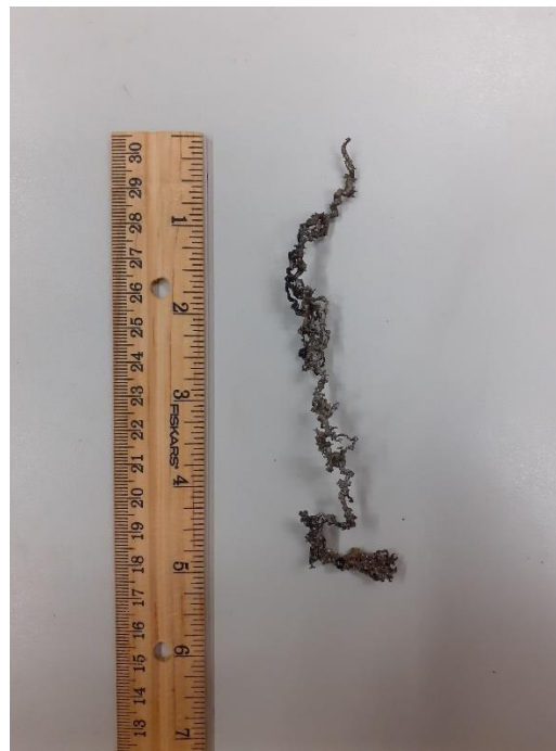
Figure 6.35: Image of casted wormhole of core 3
