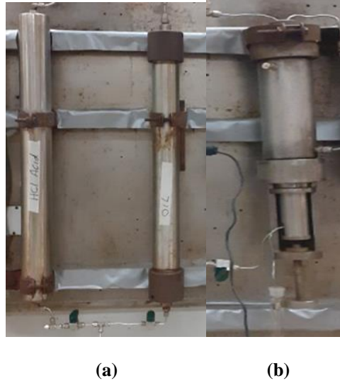
Figure 6.6: (a) Acid and oil accumulators (b) Core holder
