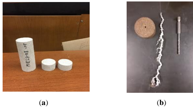
Figure 5.3: Core preparation. (a) Core is cut and drilled; (b) the 1/16-in.-drill bit used to simulate a wormhole
