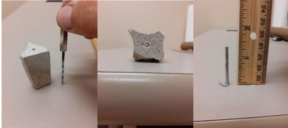
Figure D.2: Drilling a piece of core and casting it
