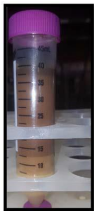
Figure 4.10: Layers of varying colors were observed when an emulsion was created using a crude oil and distilled water with the help of an emulsifier. Four distinct layers can be observed, where if the top layer is oil and the bottom layer is water, the two middle layers indicate two different emulsion layers (Oluwatosin 2016)
