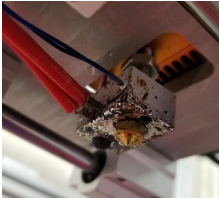
Figure 24: Clogged extruder nozzle while extruding higher composition of GF ABS
