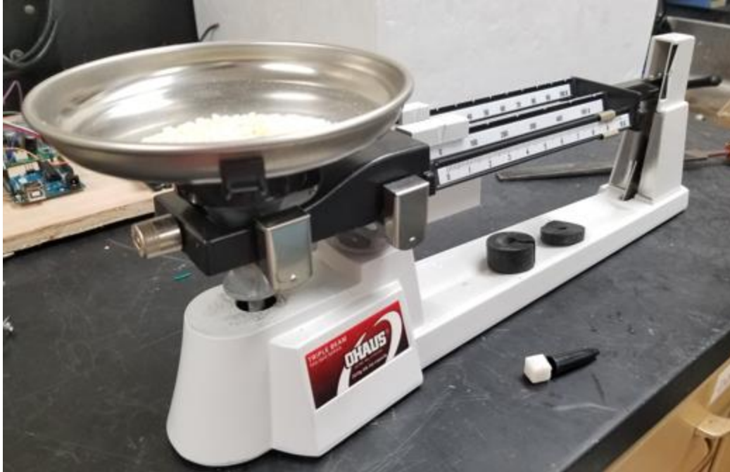
Figure 18: OHAUS beam balance weighing apparatus used for measuring the weight of pellets
