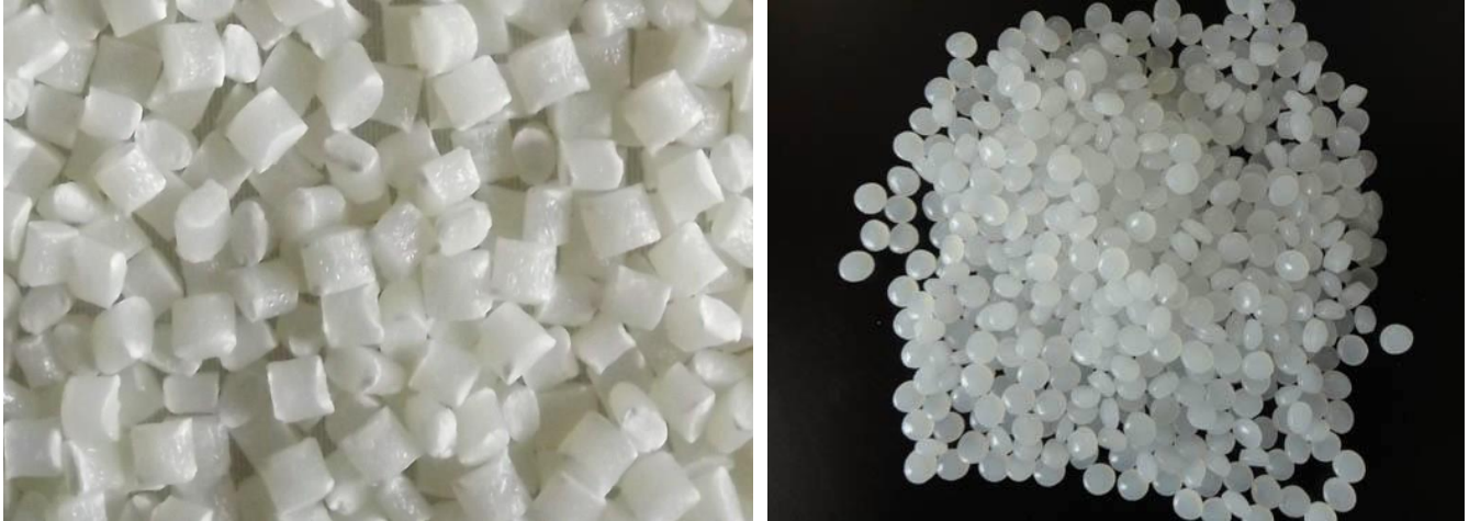
Figure 17: 30% GF ABS and LLDPE used for printing filament
