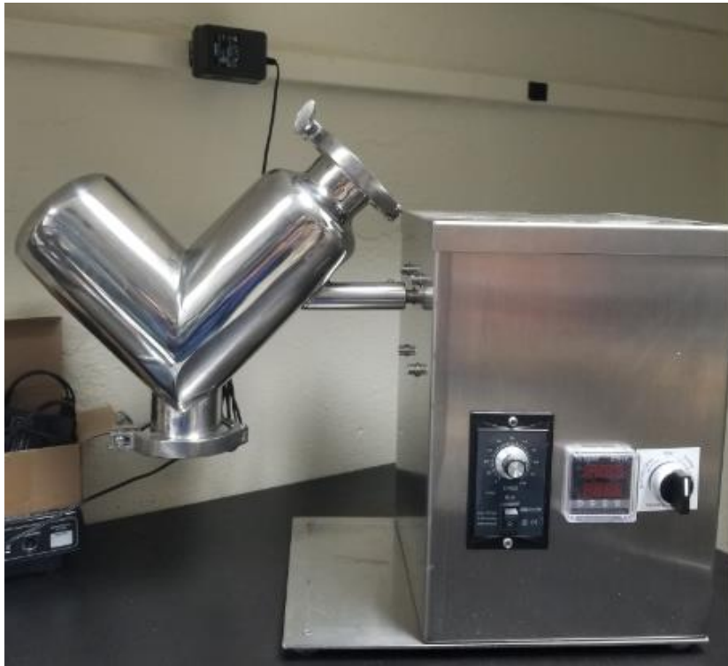
Figure 19: V-shaped mixing chamber used for mixing the calculated amount of pure ABS and 30% GF ABS
