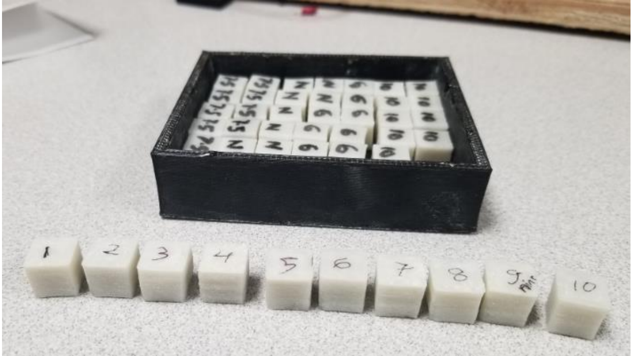
Figure 22: Test samples of dimension 10*10*10 mm to determine the young's modulus
