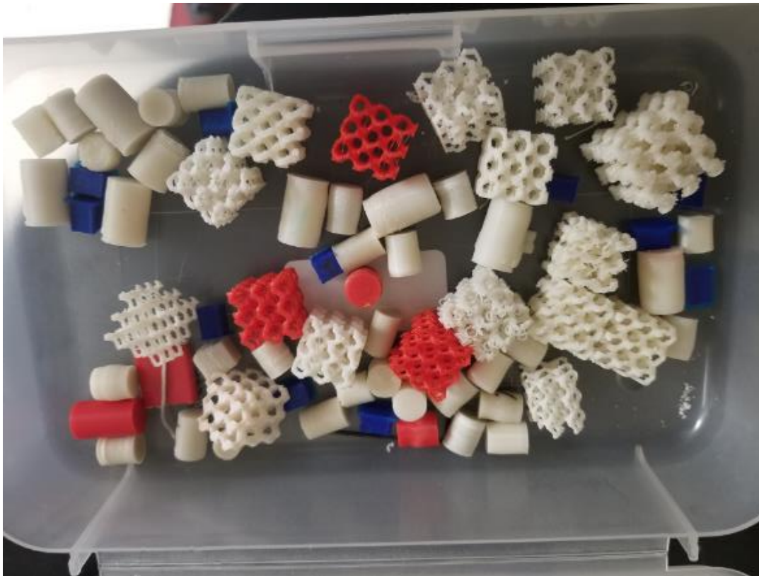
Figure 26: Various samples of different geometry printed before printing a usable test sample
