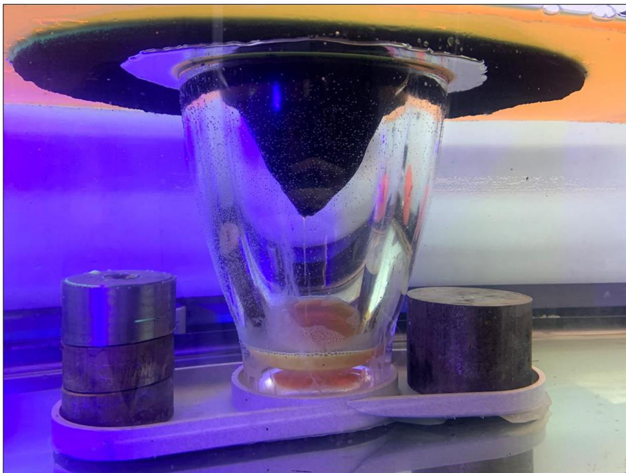
Figure A.21: A picture of the nanocomposite sponge funnel demonstrating the gravity-driven oil/water separation capabilities in a simulated gasoline spill in water.
