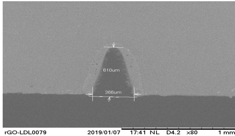
Figure 2-35 Speed 10mm/sec, Power 20% of total power, pass 1 current 20mA focal distance between lens and substrate 0.30 Cm
