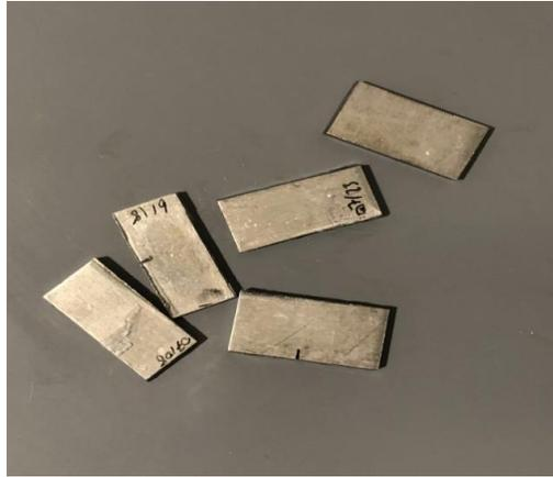
Figure 3-3 Titanium Flat samples
