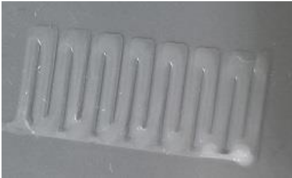
Figure 3.18: RECTANGULAR FIRST LAYER WITH INCREASED THICKNESS
