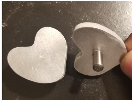
Figure 2-6: Tibia Tray Machined Using CNC Machine
