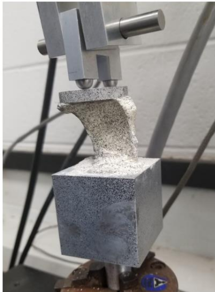
Figure 3-3-11: Mounting of the Sample on Compression Test Machine
