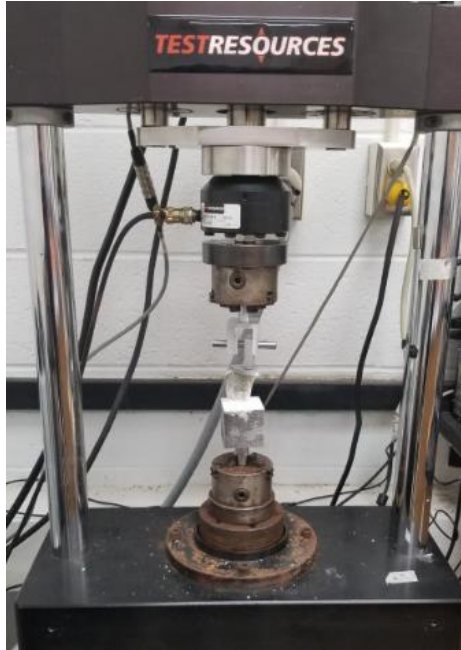
Figure 3-12: Complete Setup of the System for Fatigue Test
