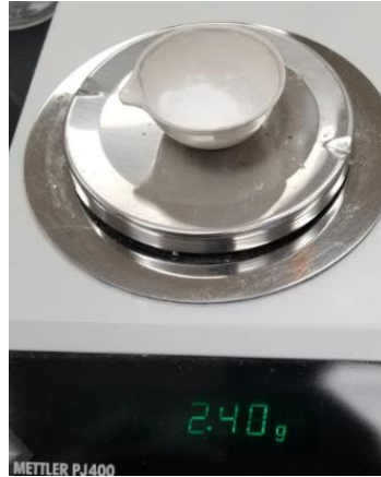
Figure 3-9: Preparation of 2.40g of PMM Cement
