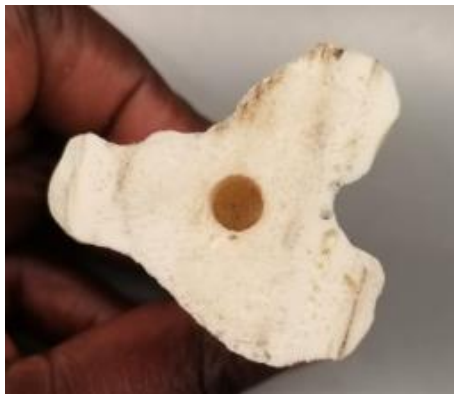
Figure 3-8: Tibia Fibula Bone with a Hole to Accommodate Tibia Tray.
