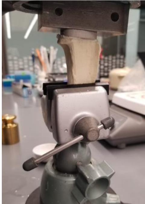
Figure 3-10: Fixation of Implant into The Bone
