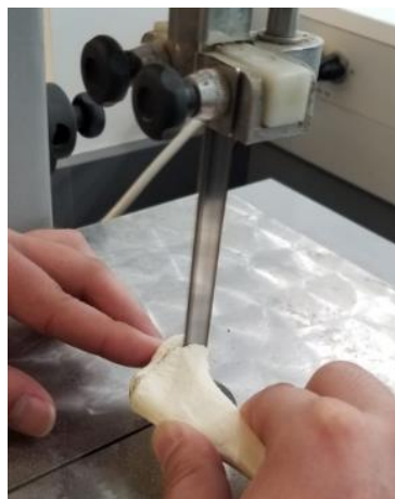
Figure 3-6: The Process of Cutting the Sawbone
