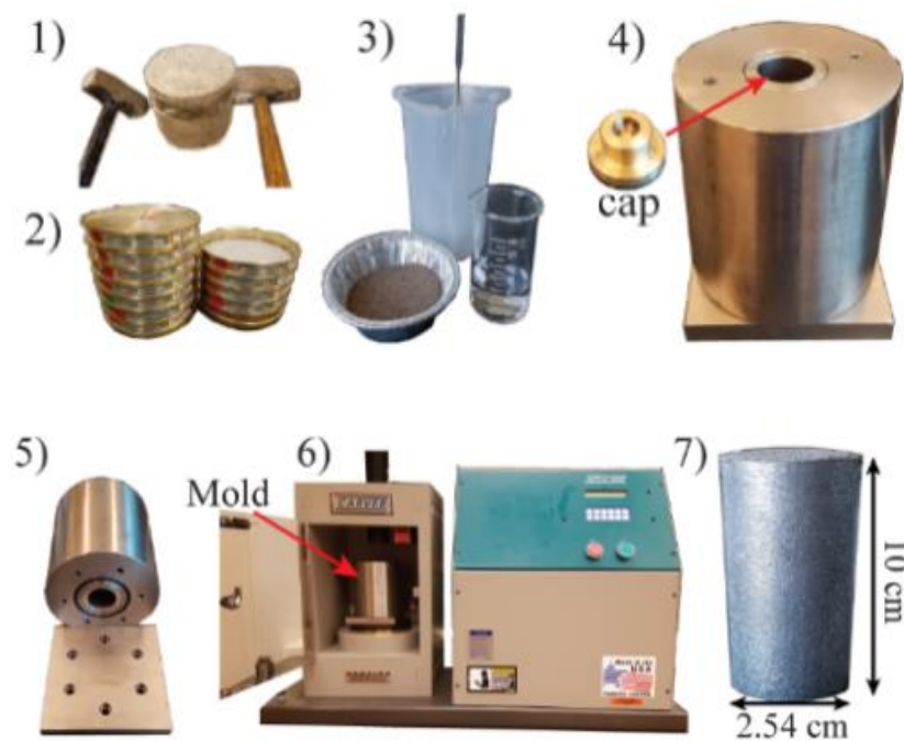
Fig 2. 5. Uniform synthetic core plug preparation: (1) Powdering dolomite rocks, (2) Sieving, (3) Mixing with deionized water, (4) and (5) Front and bottom views of the
