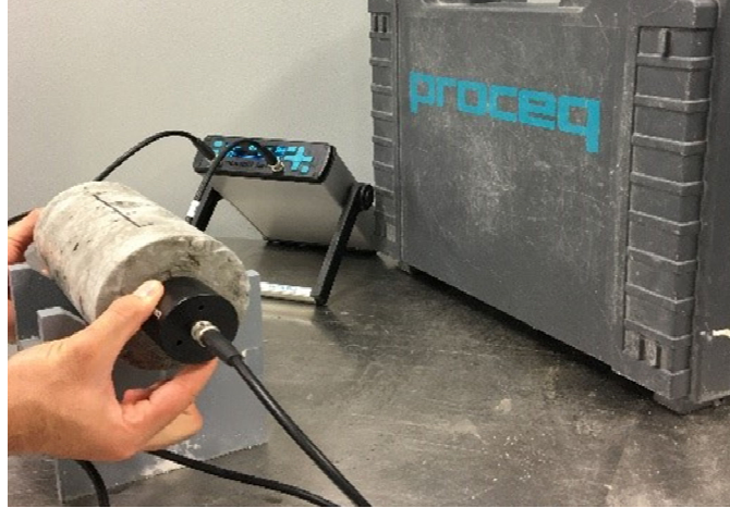
Figure 4.8: UPV Test Setup
