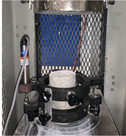
Figure 4.6: Modulus of Elasticity Test Setup
