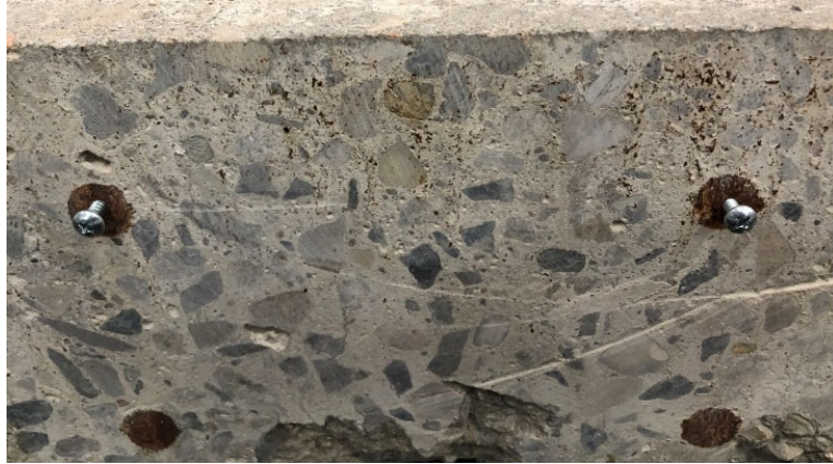
Figure 4.4: Example of Rebar Connection Using Screws
