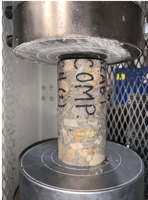
Figure 4.5: Compression Test Setup
